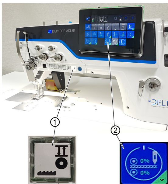
Fig. 25: Activating the puller feed drive
