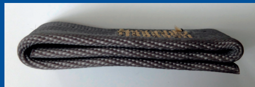
six-ply sewing for seatbelt
