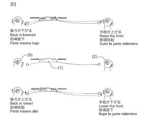
The height of the feed dog (1) will change after the angle has been adjusted. It will be necessary to re-adjust the height of the feed dog (1).
