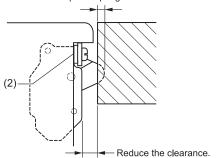
If further adjustment is necessary, add another washer of the same thickness.
