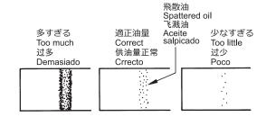
**5** Check the amount of oil which has spattered onto the sheet.
