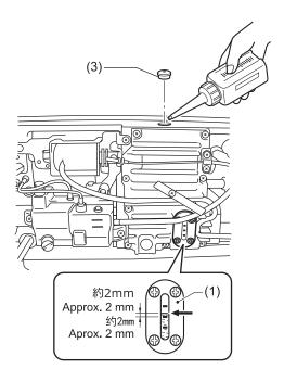
Add lubricating oil until the oil level is approximately 2mm above the center reference line in the oil window (1).
