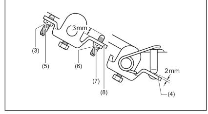
13 Turn the screw (7) until the distance between the end of the screw (7) and the knee lifter (8) is approximately 3mm.
