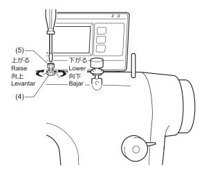
4 Use a screwdriver to turn the adjustment screw (5) to adjust the floating amount.
