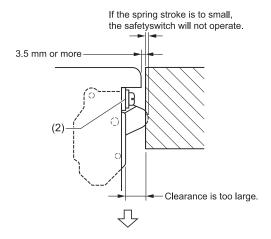
By changing the position of the safety switch, the required spring stroke can be maintained.
