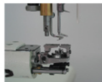
differential feed as standard "no wave" finish
