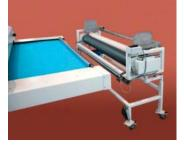
Our Laminating system can be equipped with: 3 Position Unwinding = FABRIC + FILM + FABRIC 2 Position Unwinding = FABRIC + INTERLINING
