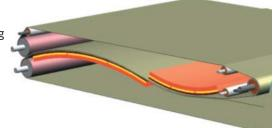
C40 inner core body with 2 different vulcanized silicon hardness covers.
