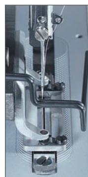
Position of the needle bar during sewing
