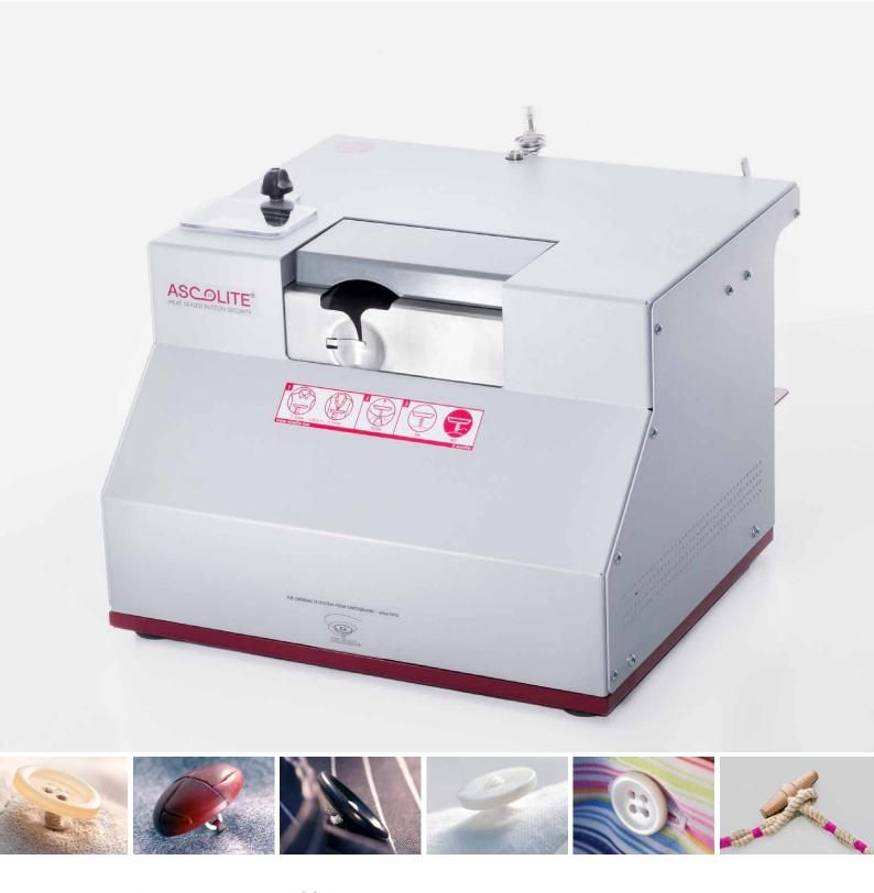
The fully automatic BSS-MK13 is designed to wrap and to secure all types of sewn buttons at high and constant precision.
