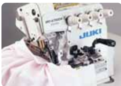
● Gathering MO-6714DA-BE6-327/S162 (S162: Swing-type gathering device, manual-lever operated)
