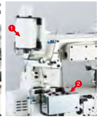
1 Presser lifter drive mechanism magnet 2 Thread trimmer drive mechanism magnet
