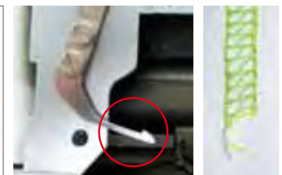
New cloth guide / The new cloth guide helps the machine perform hemming while keeping the hem width consistent.
