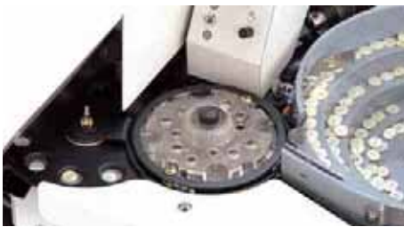
● Horizontal, forced feed mechanism
