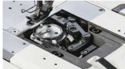
② Bed slide with an open/close sensor
