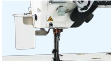
① Eye guard with an open/close sensor
