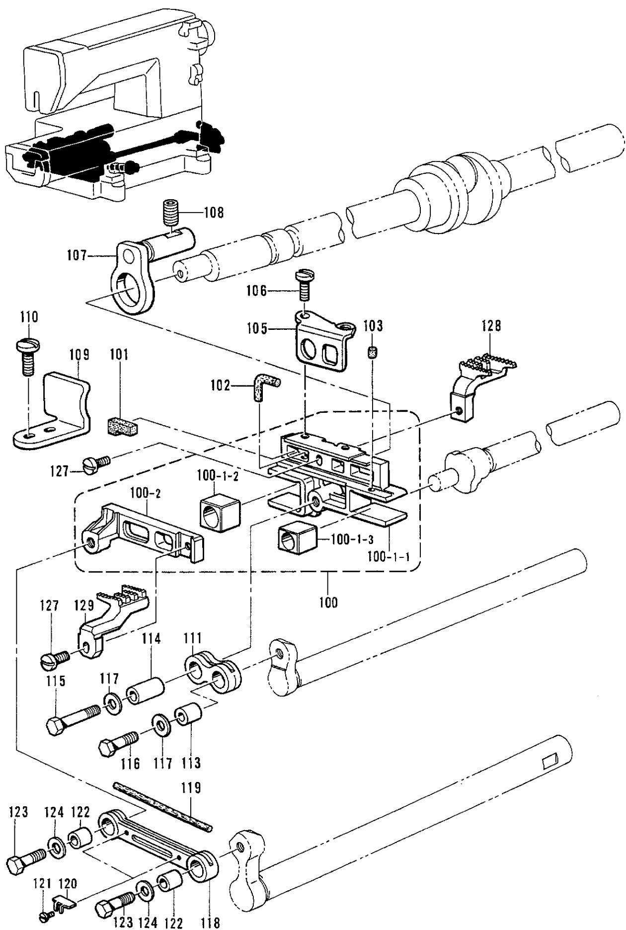
E2. 送り関係/Feed mechanism/Transportvorrichtung/
