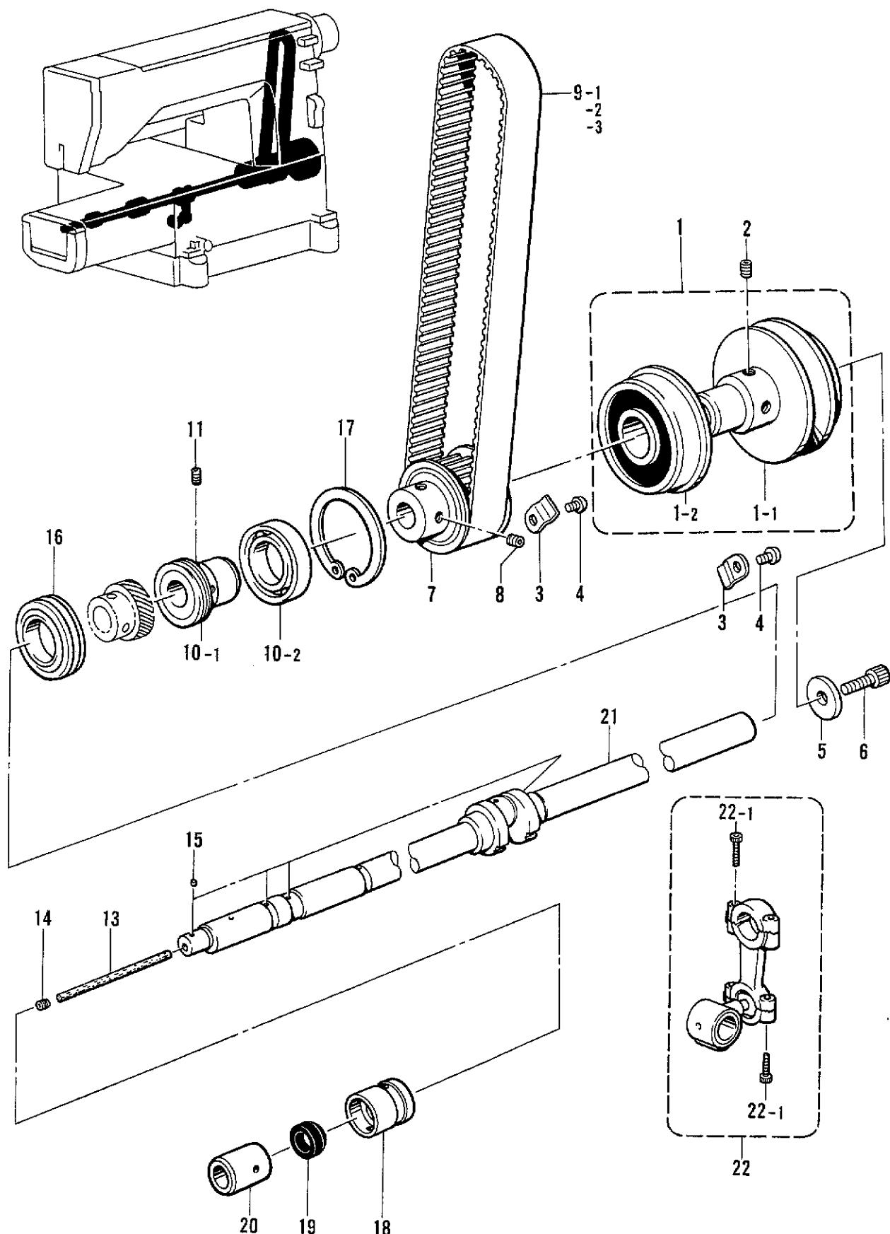
F. 下軸関係/Lower shaft mechanism/Untere Welle/
