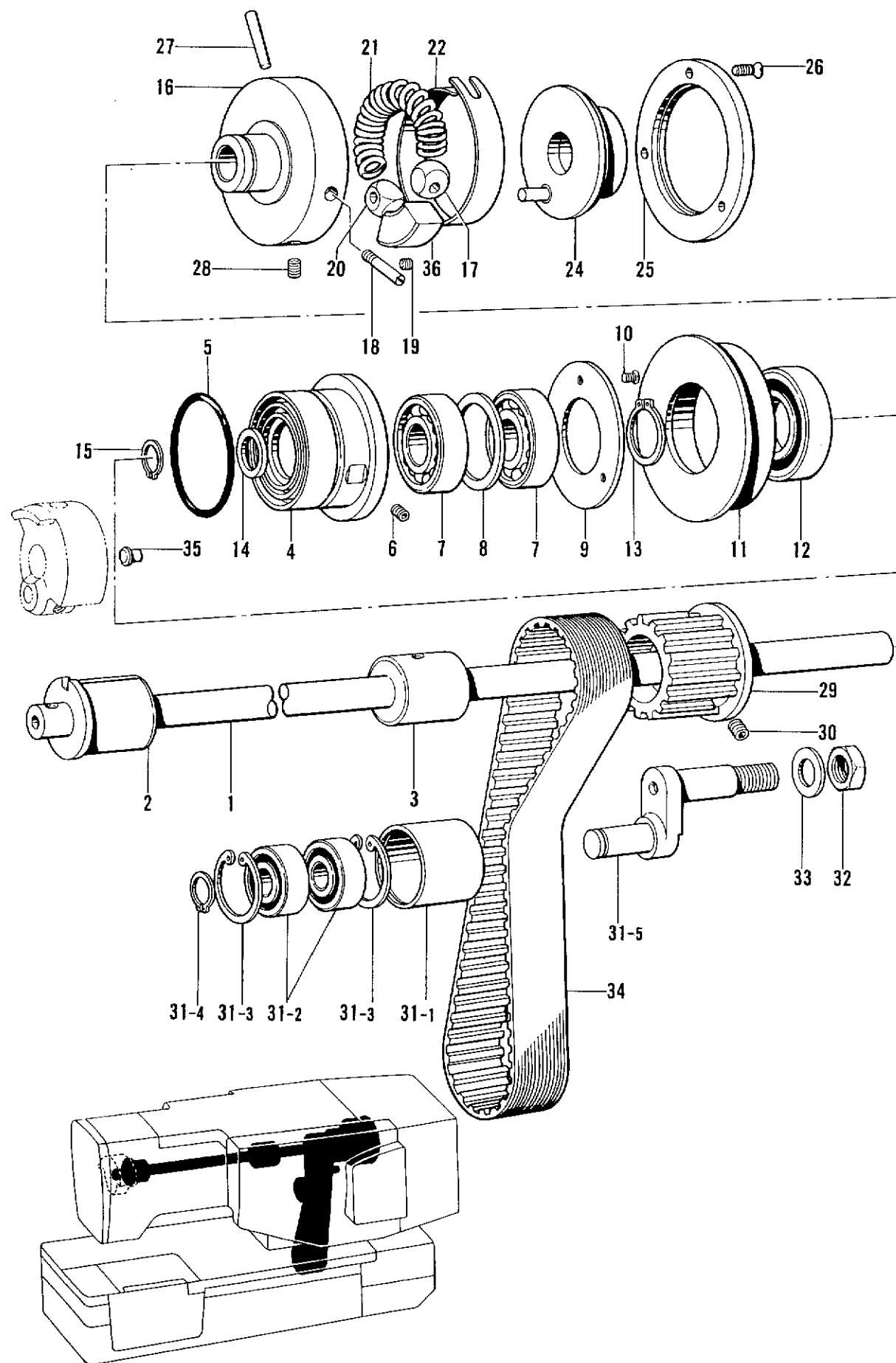
B. 上軸関係 /Upper shaft mechanism /Obere Welle /
