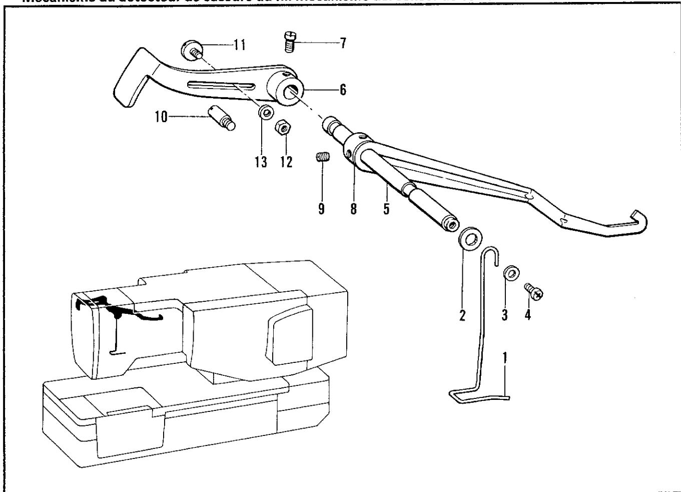
Q. 下軸関係 / Lower shaft mechanism / Untere Welle /
