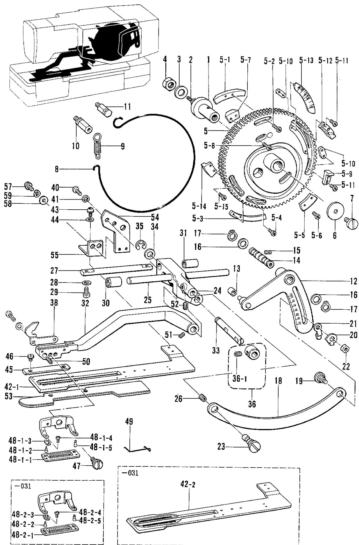
M. 送り関係/Feed mechanism/Transportvorrichtung/
