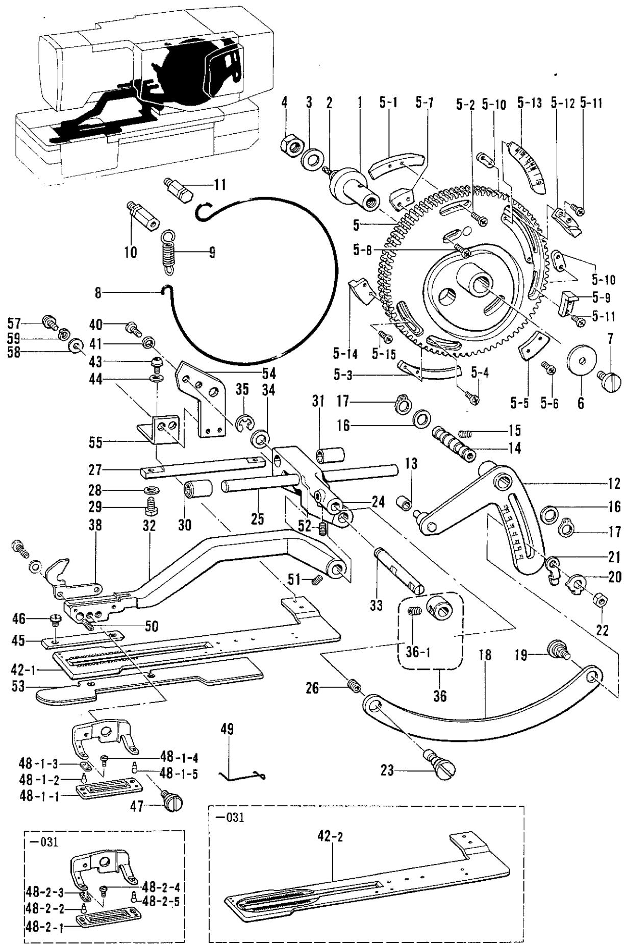
M. 送り関係/Feed mechanism/Transportvorrichtung/
