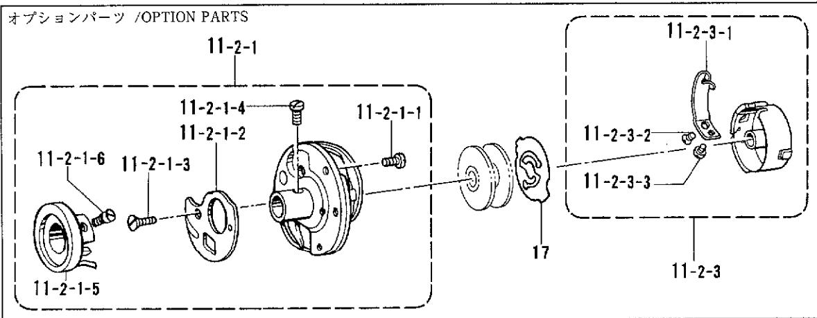
R. カマ関係/Rotary hook mechanism/Greifervorrichtung/
