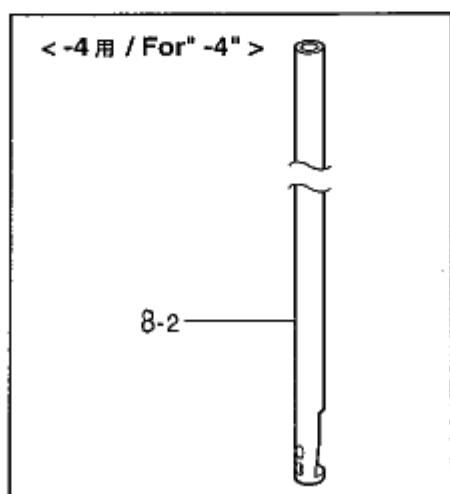
B . 針棒・天秤関係 / Needle bar and thread take-up mechanism
