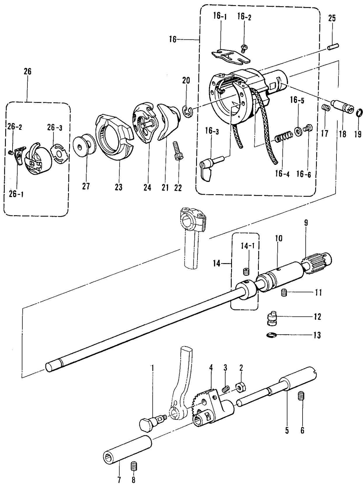
G. 下軸関係/Lower shaft mechanism/Untere Welle/
