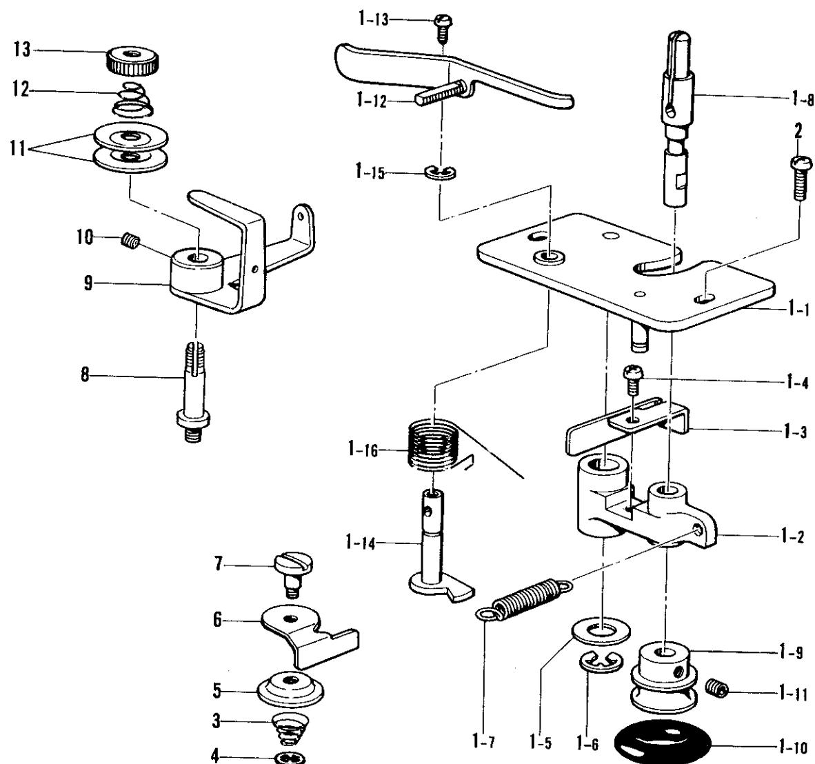
K. 糸巻関係/Bobbin winder mechanism/Spuler/
