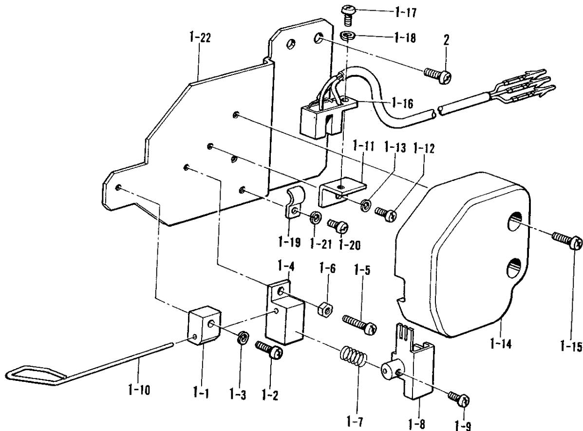
Q. 糸切れ感知関係/Thread breakage detector mechanism/Fadenbruchfühler/
