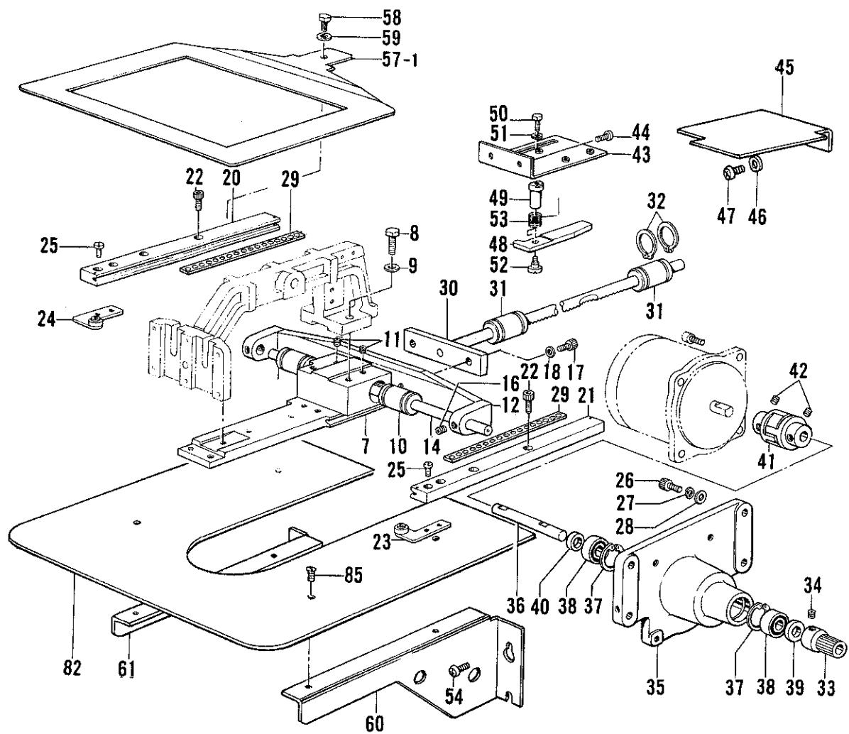
D2. 送り関係/Feed mechanism/Transportvorrichtung/
