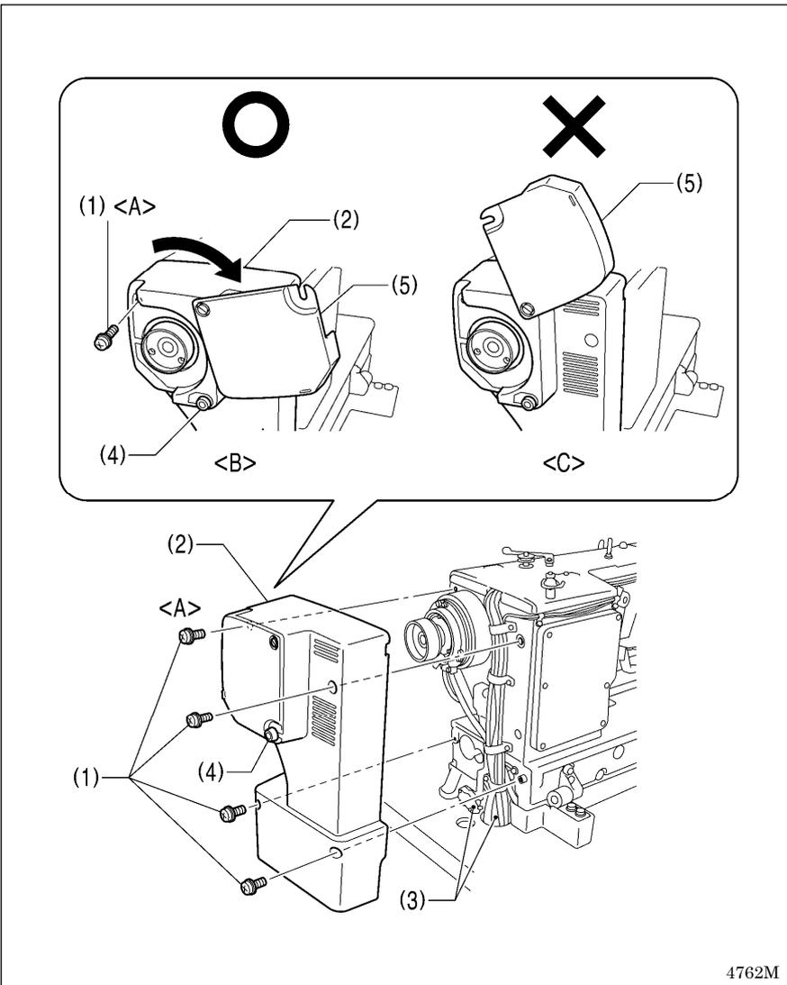
1. Install the motor cover (2) with the three screws (1) (other than <A>).
