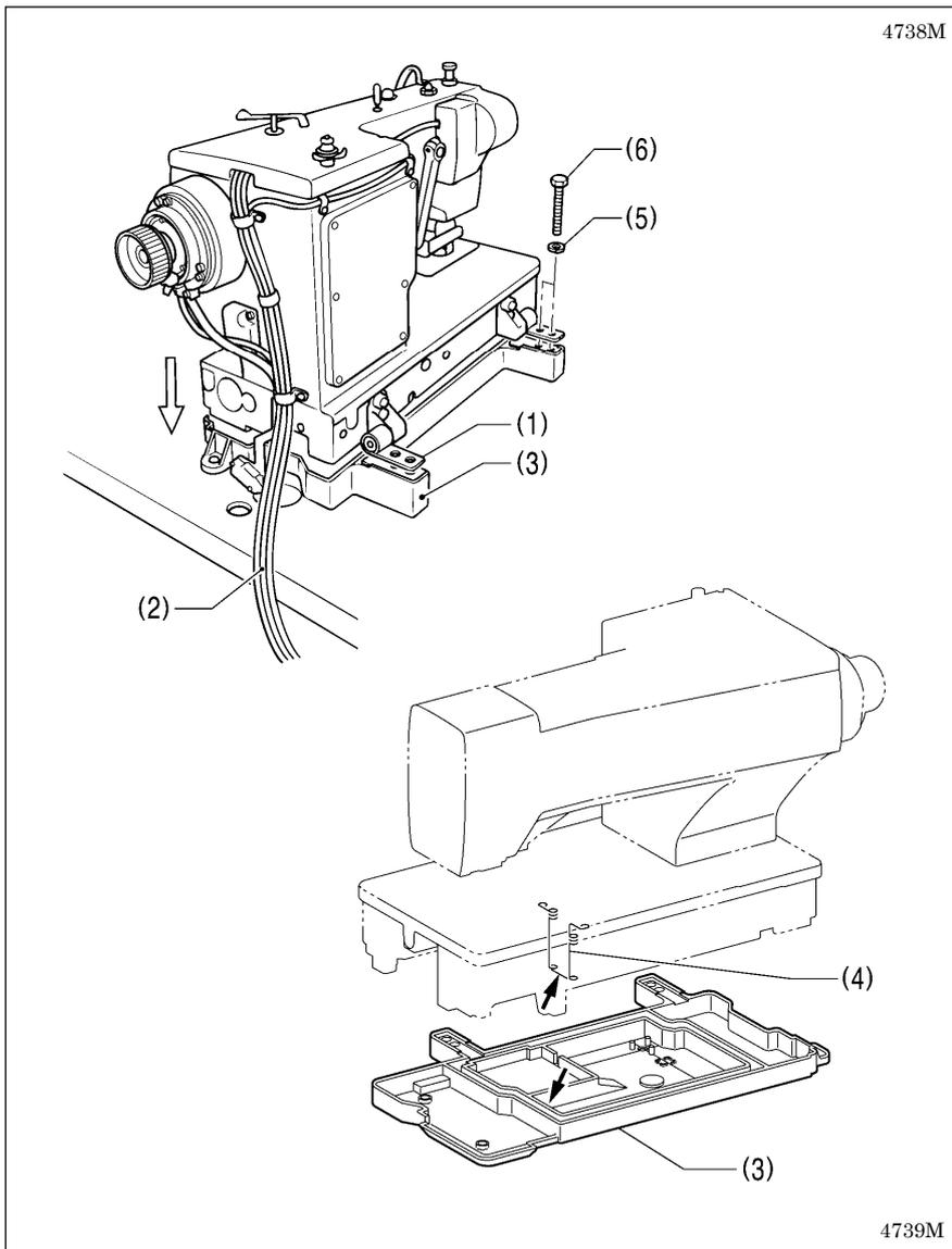
1. Place the two bed hinges (1) so that they are level as shown in the illustration at left, and then place the machine head gently on top of the bed base (3) so that the cables (2) do not get clamped.
