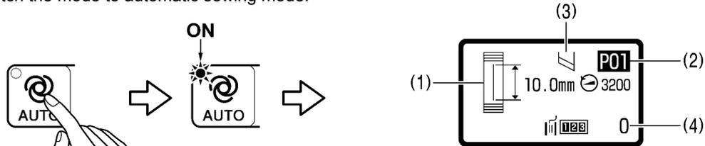
Information such as the sewing pattern (1), the program number (2), the cutter operation (3) and the lower thread counter (4) will appear in the display.
