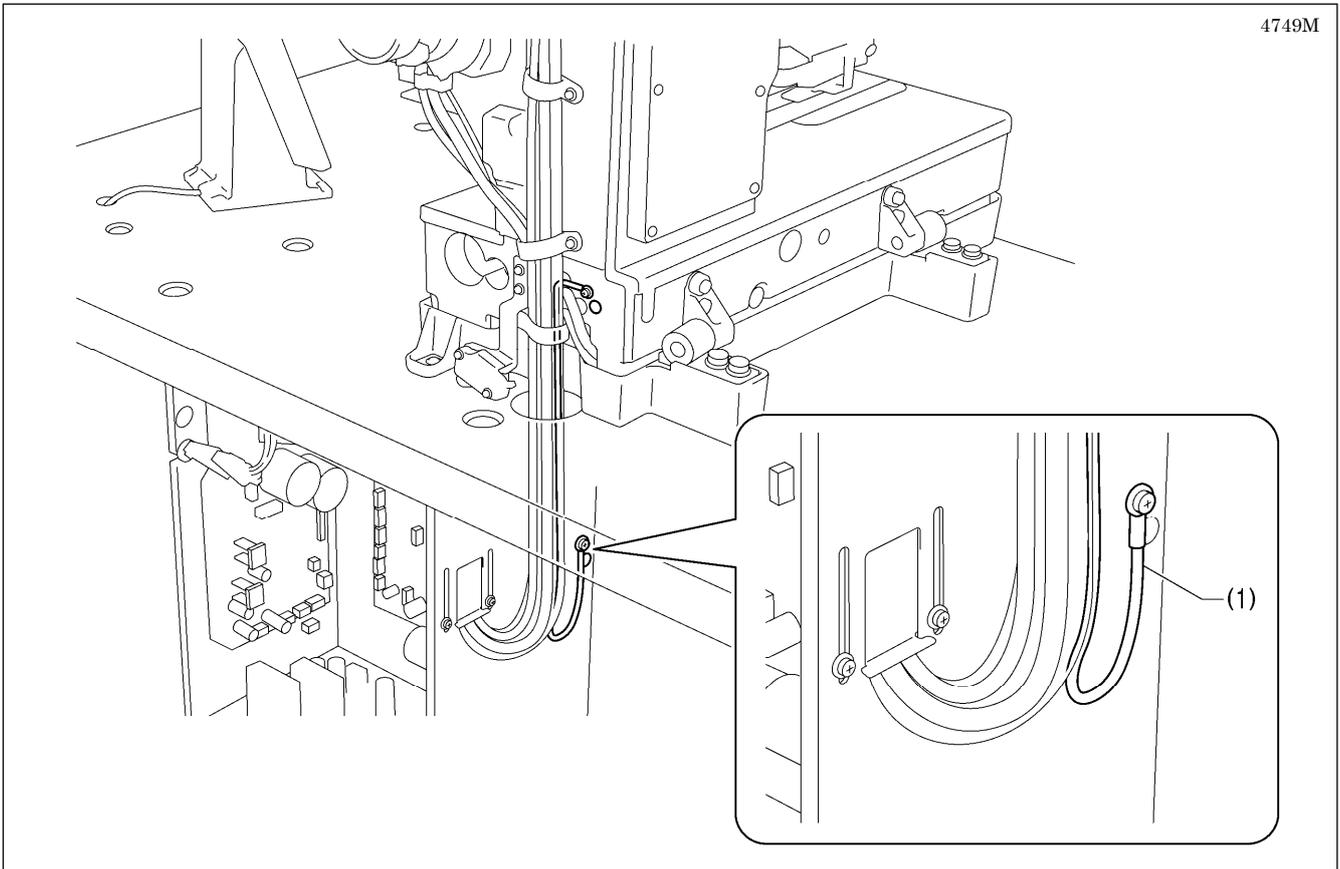
(1) Ground wire from the machine head (Ground mark position)
