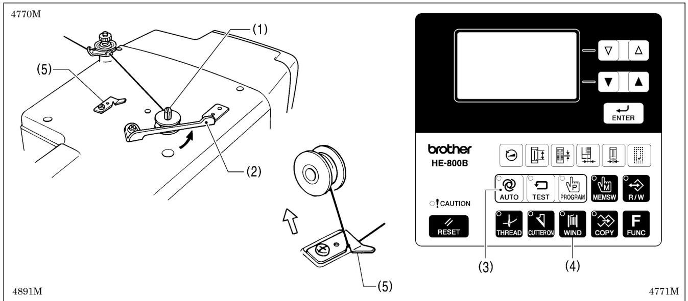
1. Place the bobbin onto the bobbin winder shaft (1).
