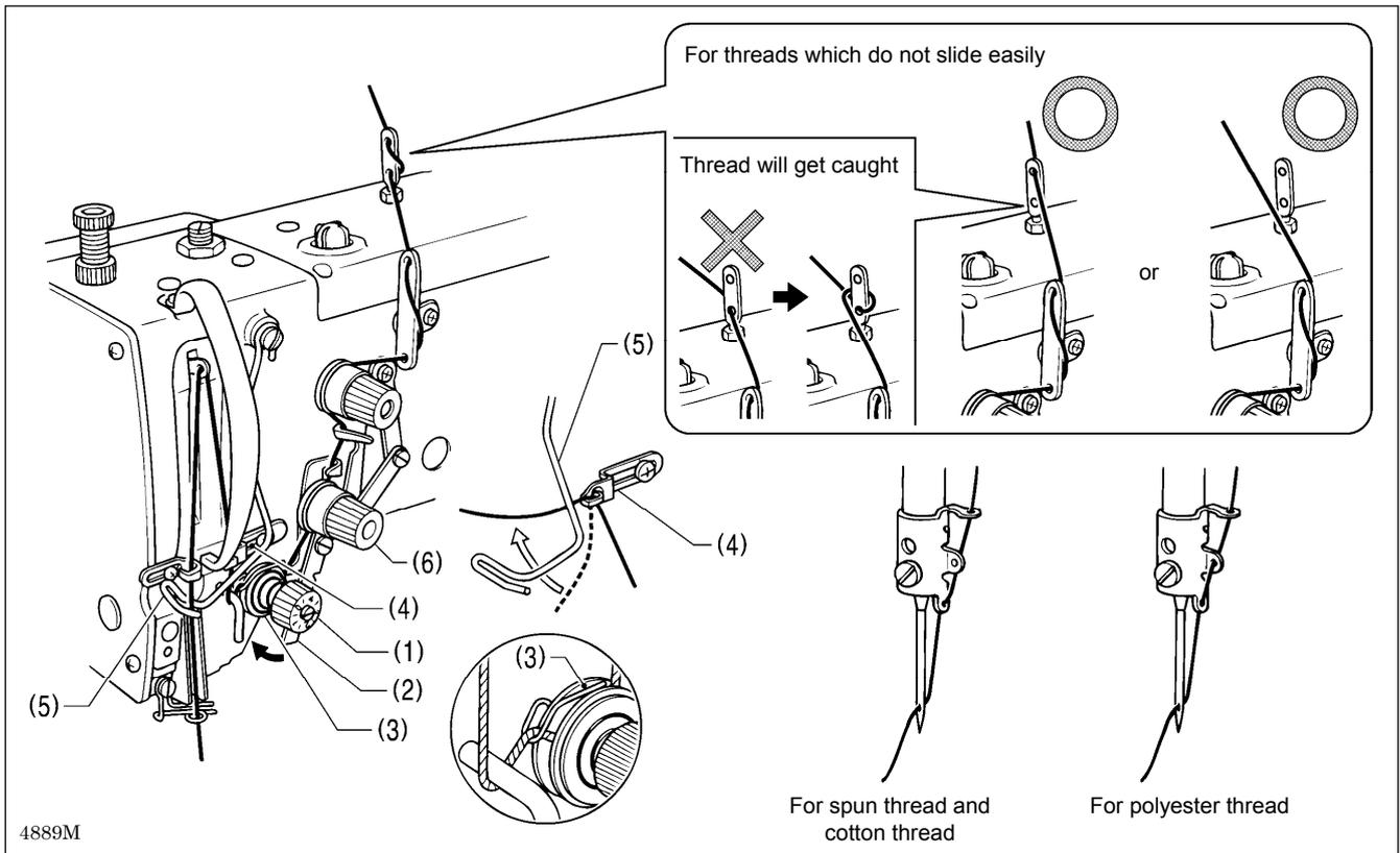
Thread the upper thread correctly as shown in the illustration.
