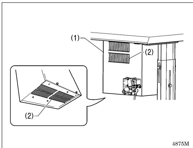
Use a vacuum cleaner to clean the filter in the air inlet port (2) of the control box (1) at least once a month.
