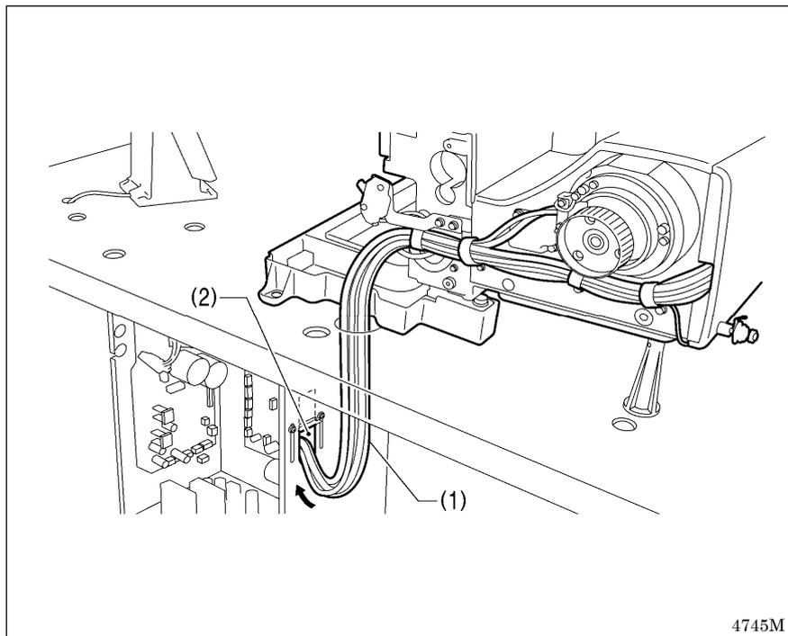
1. Pass the cord bundle (1) through the hole in the work table.
