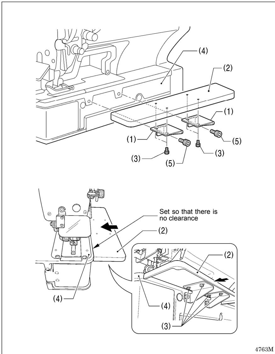
1. Provisionally install the two table support plates (1) to the auxiliary table (2) with the four bolts (3).
