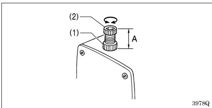
The standard distance A is 30 mm (approximately 30 N). Loosen the nut (1) and turn the adjusting screw (2) to adjust the work clamp pressure.
