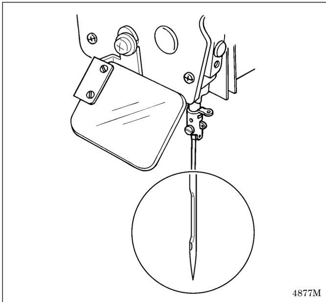
Always check that the tip of the needle is not broken and also the needle is not bent before starting sewing.
