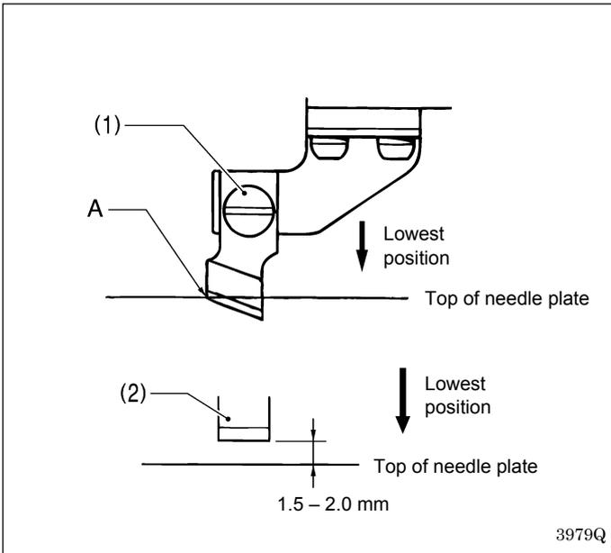
1. Install the cutter with the screw (1) so that the tip A of the cutter blade is aligned with the top of the needle plate when the cutter is pressed down by hand to its lowest position.
