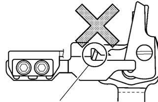
Install so that the projection on trimmer M is not inserted.
