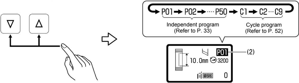
The program number (2) changes in the order shown in the illustration each time the  $\Delta$  key is pressed. (The  $\nabla$  key changes the order in the opposite direction.)
