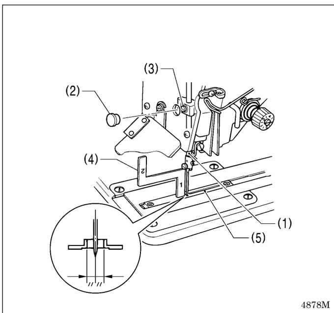
1. Press the THREAD key to switch to threading mode.
