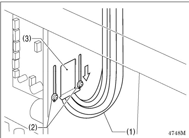
4. Close the cord presser plate (3) in the direction of the left arrow, and secure it by tightening the two screws (2).
