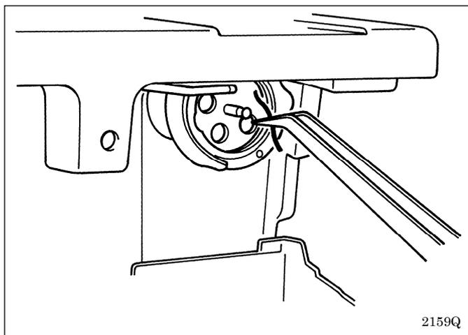
3. Remove the bobbin case, and remove dust and lint from around the shuttle and fixed knife.
