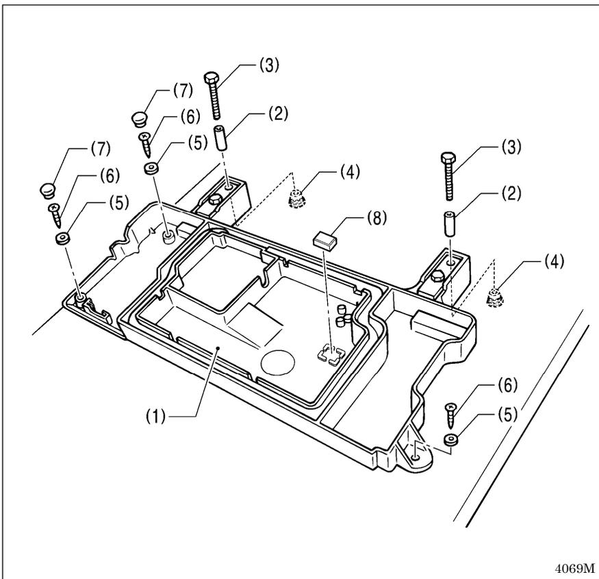
1. Place the bed base (1) on top of the work table, and insert the four collars (2).
