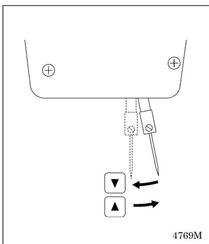
If you press the ▼ key while in threading mode, the needle will return to the middle position.
