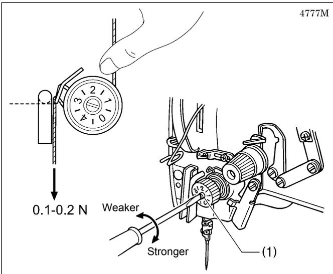
Turn the thread tension stud (1) to adjust the thread take-up spring tension to between approximately 0.1 - 0.2 N in accordance with the material to be sewn.
