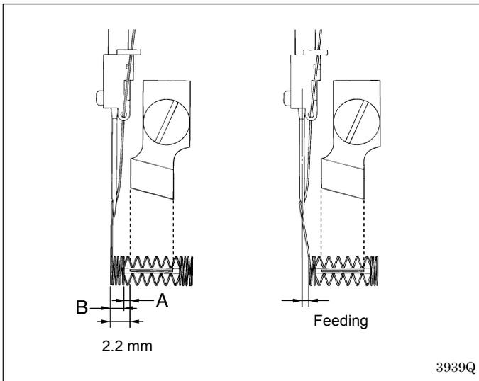
Because the needle and cutter positions are separated by 2.2 mm as shown in the illustration, the distance between the edge of the front tuck and the edge of the buttonhole cannot be set to less than 2.2 mm.
