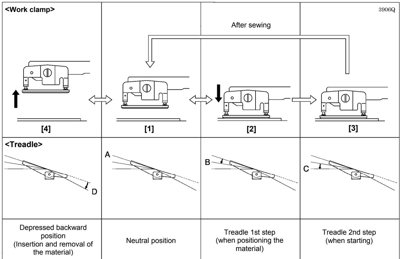
1. When the treadle is not depressed (A), the work clamp is at the neutral position. (Figure [1])
