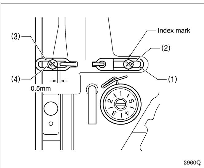
The standard position of arm thread guide (1) is when the screw (2) is aligned with the index mark. The standard position for the arm thread guide (3) is when the clearance between it and the screw (4) is 0.5 mm as shown in the illustration.
