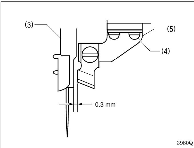
2. Loosen the two screws (4), and move the cutter holder (5) to adjust so that the clearance between the cutter and the needle bar (3) is 0.3 mm.
