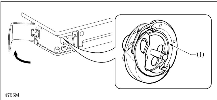
When first installing the machine and when the machine has not been used for an extended period of time, remove the bobbin and add 2-3 drops of oil to the rotary hook race (1) before sewing.
