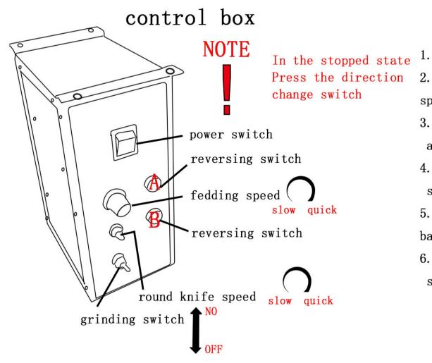
1. power switch:Control box power switch 2. fedding speed:Feed wheel adjustment speed
