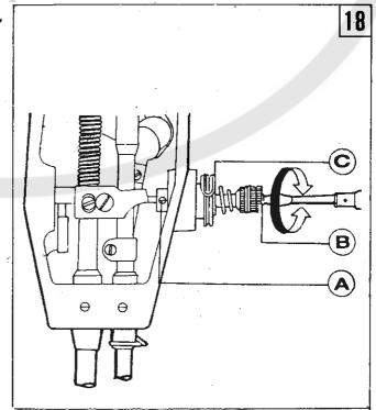
2) Adjusting the sewing range of thread take—up spring (Fig. 19)
