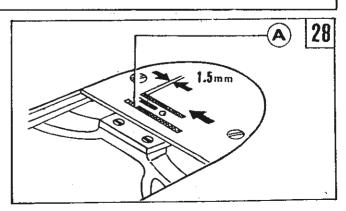
To adjust the position of feed dog, move feed doy to the front end of throat plate. Loosen Screw A (See Fig 29b), move feed dog support B in the direction shown by arrow (Fig. 29a) to adjust. After adjustment tighten Screw (A).
