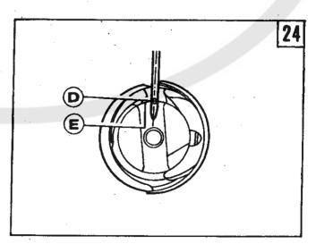
2 Adjusting rotating hook point timing with needle.
