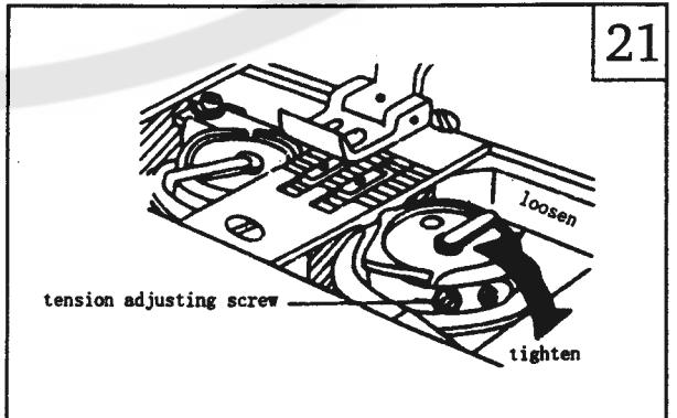
b. If the needle thread is too loose and the bobbin thread is too tight, then shows as Fig. 20C, And turn the thread tension screw clockwise to increase the needle thread tension; or turn loose the bobbin lace screw to reduce the bobbin thread tension. (See Fig. 21, 22)
