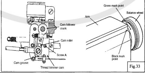
Note: To adjust, Loosen two thread trimmer cam clamp screws A.
