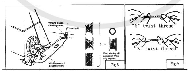
It is recommended to use "S" twist thread in the left needle (Viewed from front), and "Z" twist thread in the right needle.
