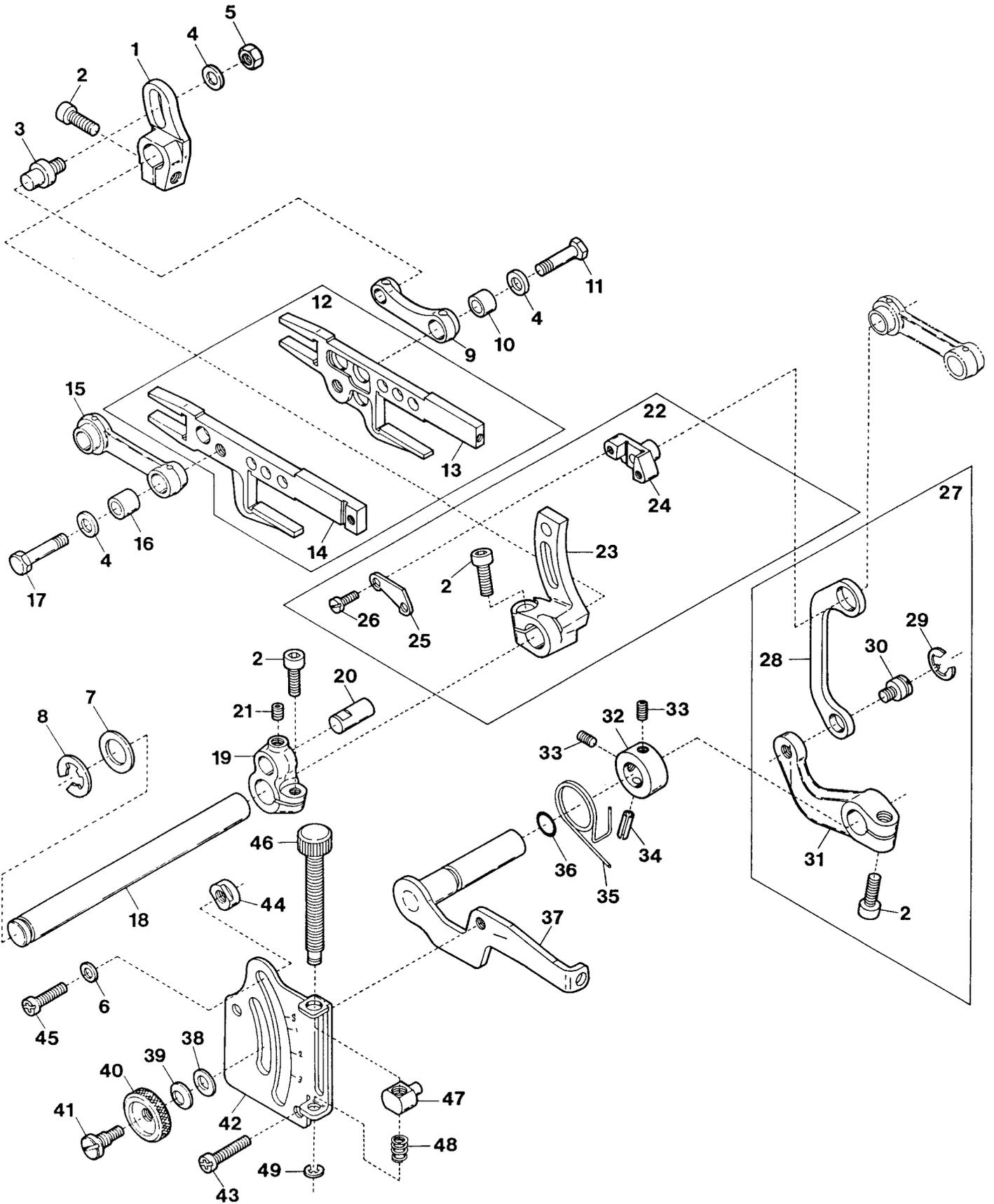
FEED DRIVING CONTROL MECHANISM
