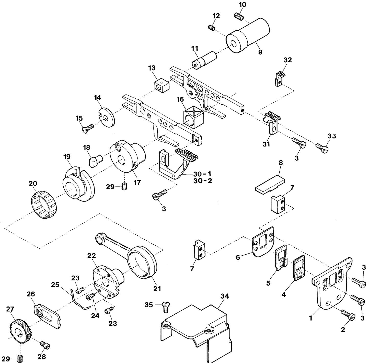
FEED DRIVING MECHANISM
