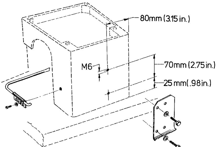
The blower device can be mounted supplementary also on former bag feed-in devices. For this, two tap holes M6 have to be drilled on the rear of the gear box of the bag feed-in device, see sketch.
