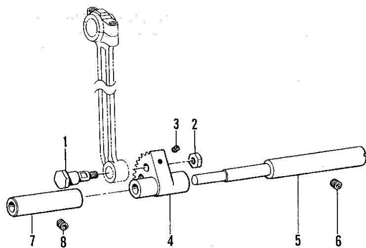
K. 下軸関係/Lower shaft mechanism/Untere Welle/
