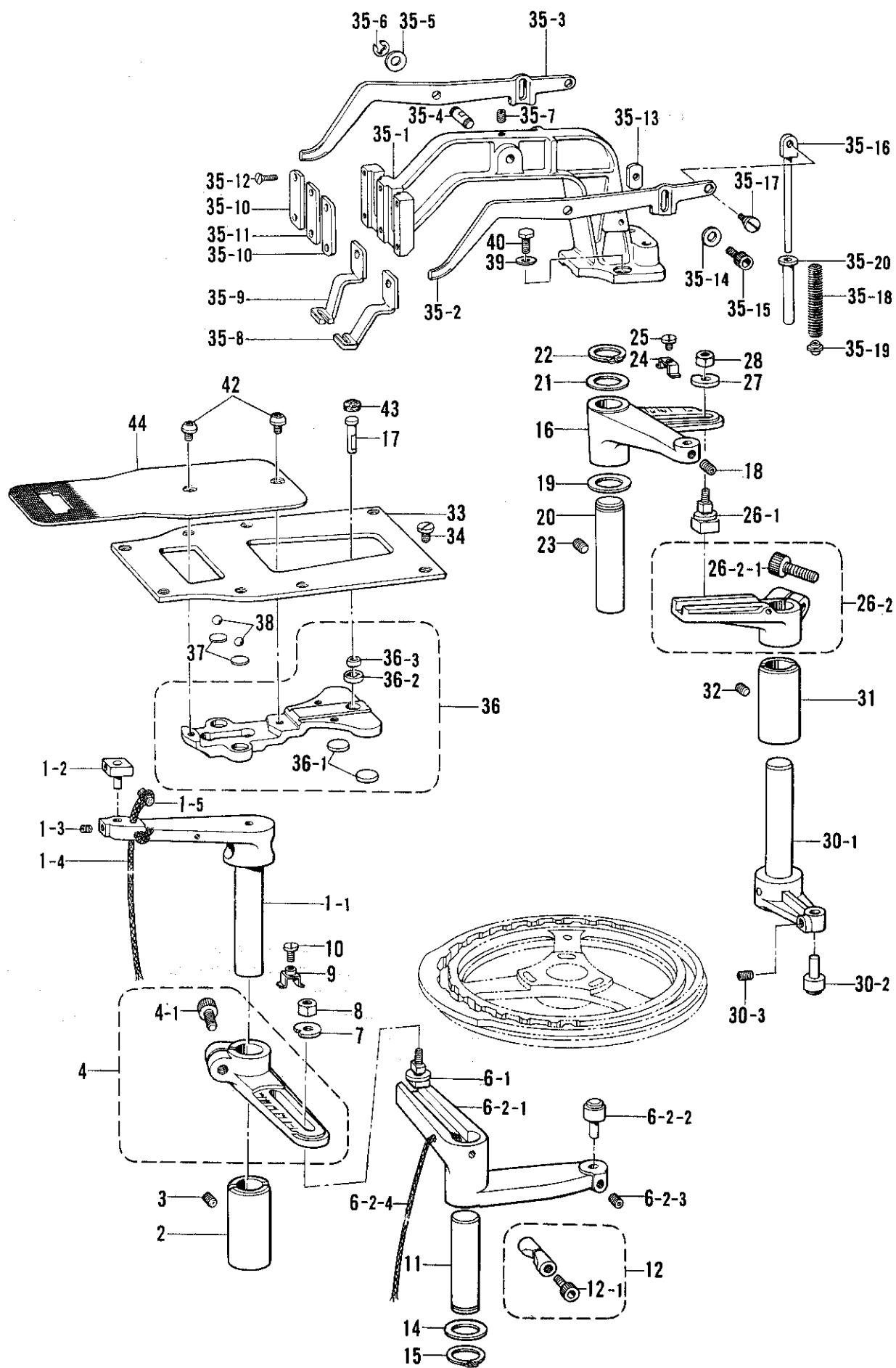
F. 送り関係/Feed mechanism/Transportvorrichtung/
