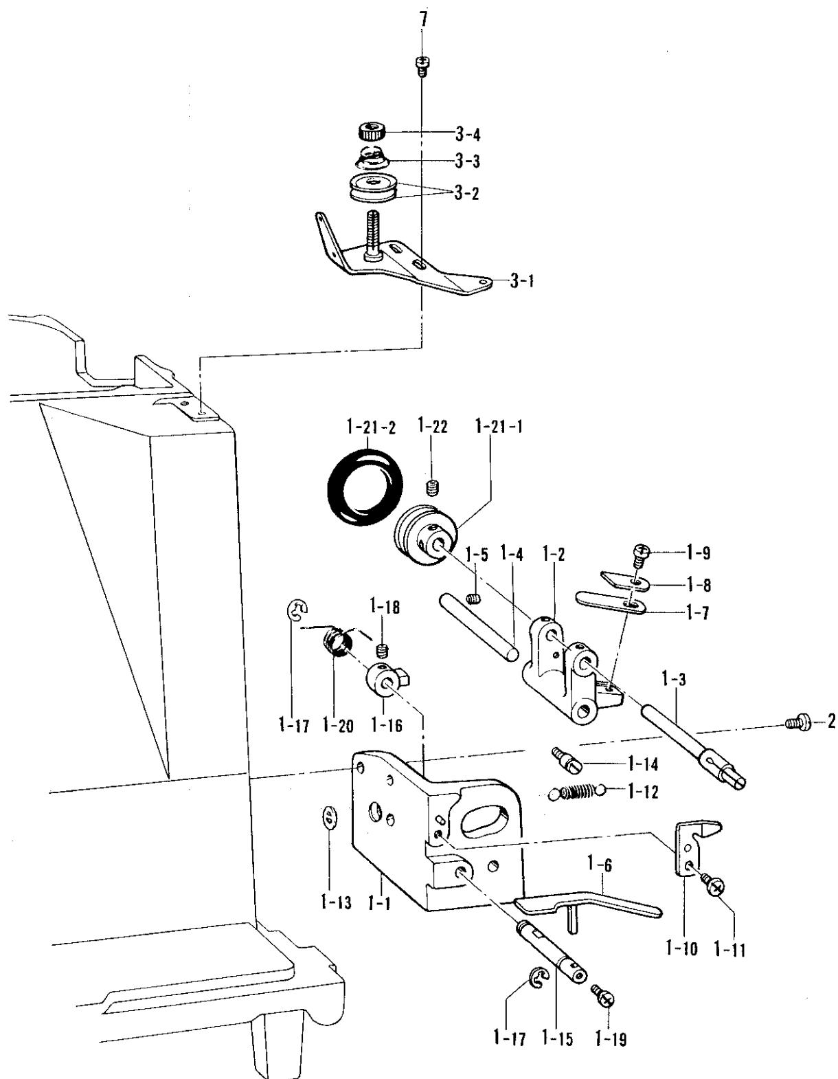
N. 糸巻き関係 / Bobbin winder mechanism / Spuler /
