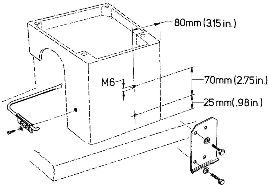
The blower device can be mounted supplementary also on former bag feed-in devices. For this, two tap holes M6 have to be drilled on the rear of the gear box of the bag feed-in device, see sketch.
