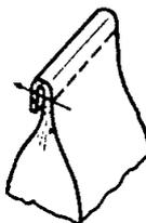
**GB(S)29910G / FB(S)29910A** Combined bag feed-in, trimming and taping device with crepe tape folder. Width of tape not adjustable. Folder available for 50, 55 and 60 mm wide tapes. Please specify. Standard 50 mm. Speed 11-23 m/min. at 50 Hz. Gear motor I = 30:1.
