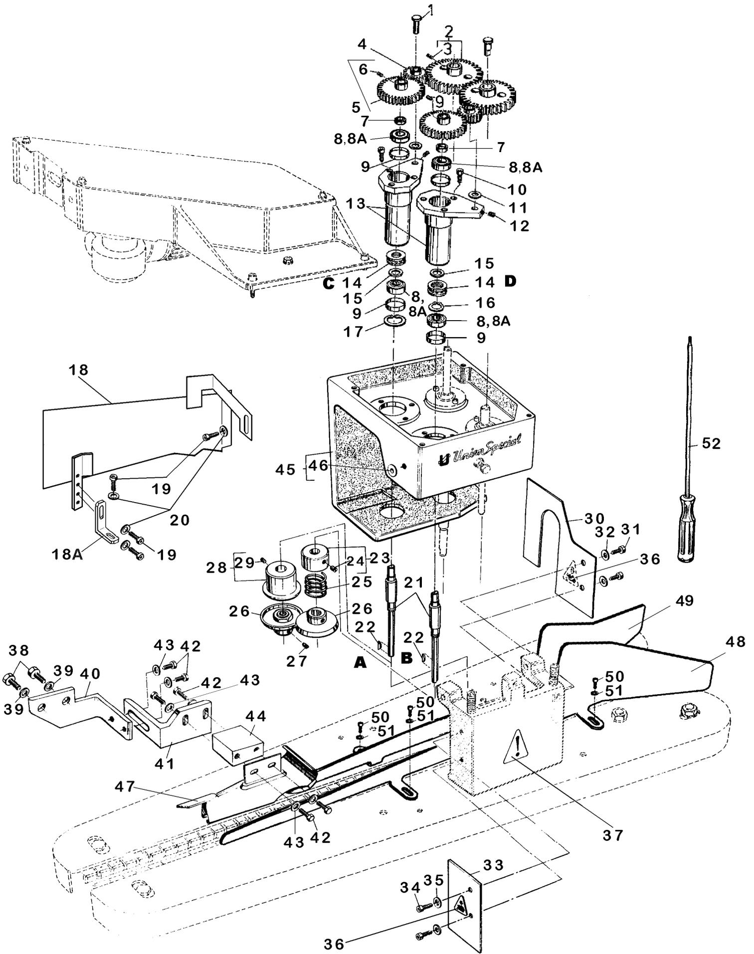
**BAG FEED-IN, TRIMMING AND TAPING DEVICE NO. 29910**
