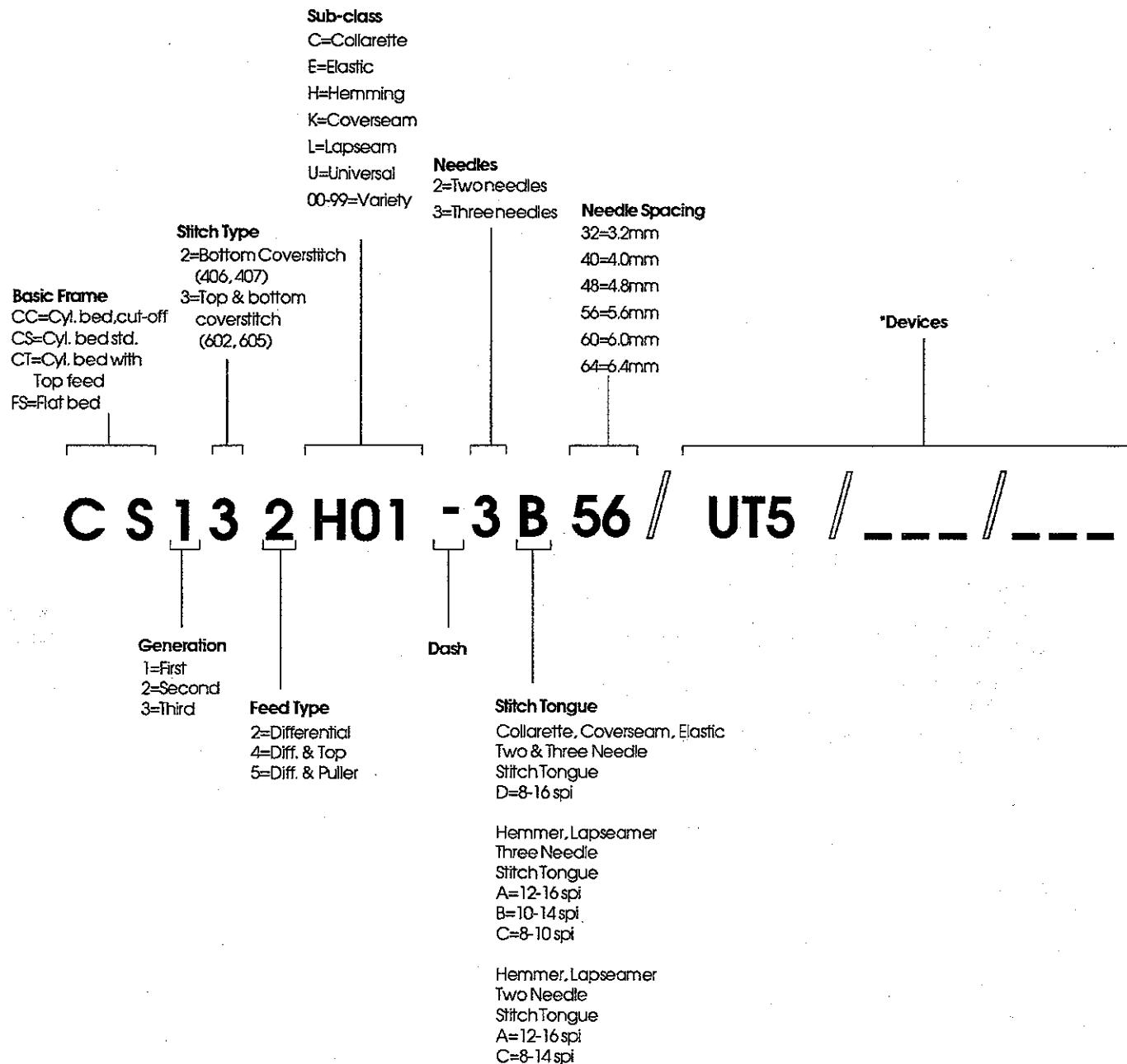
**UT4 for use on CS122 Styles** = Pneumatic (air), thread trimmer, needle thread wiper (blower) and presser foot lift assist.
