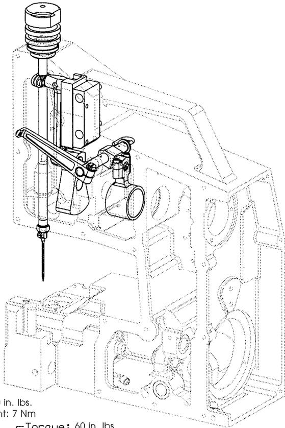
1 Seal threads with grease or liquid gasket
