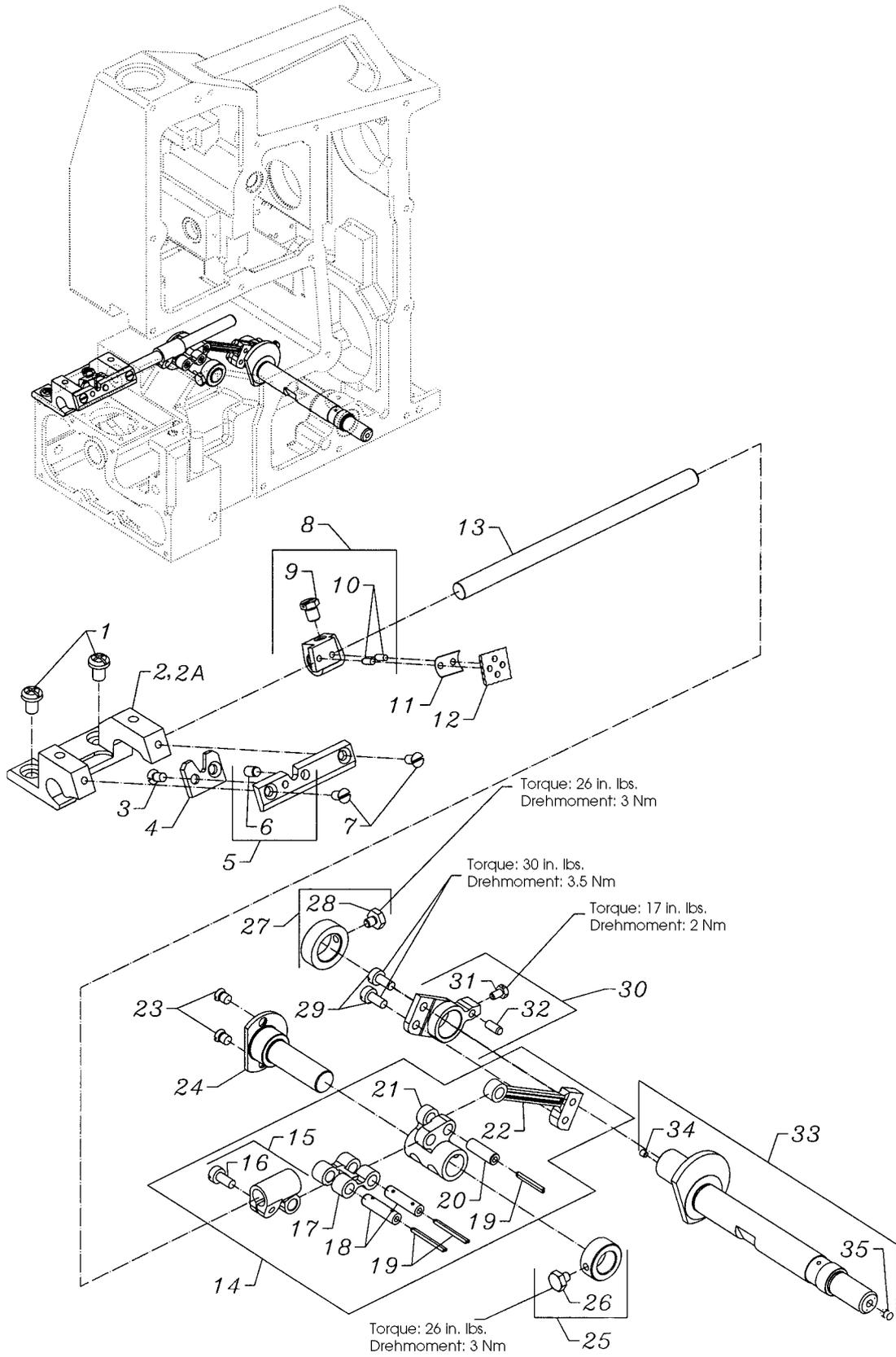
**THROAT PLATE SUPPORT, KNIFE DRIVE BM111C, BML111C**
