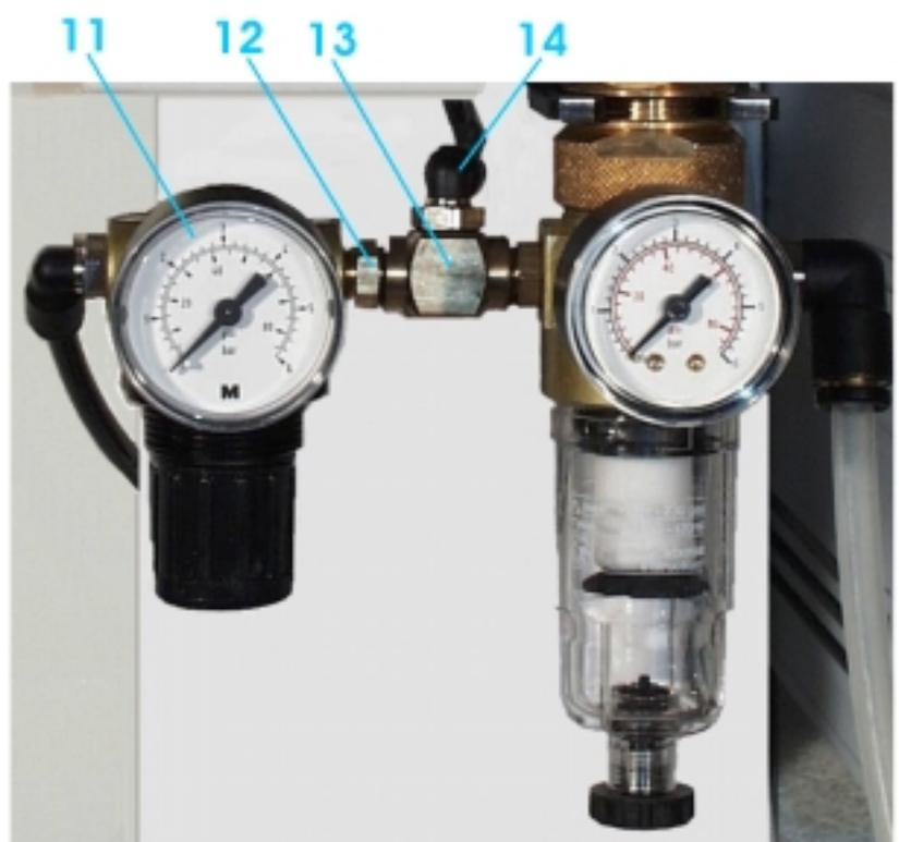
**CONTROL FOR ELECTRO-PNEUMATIC THREAD CHAIN CUTTER BM111C1, BML111C1**
