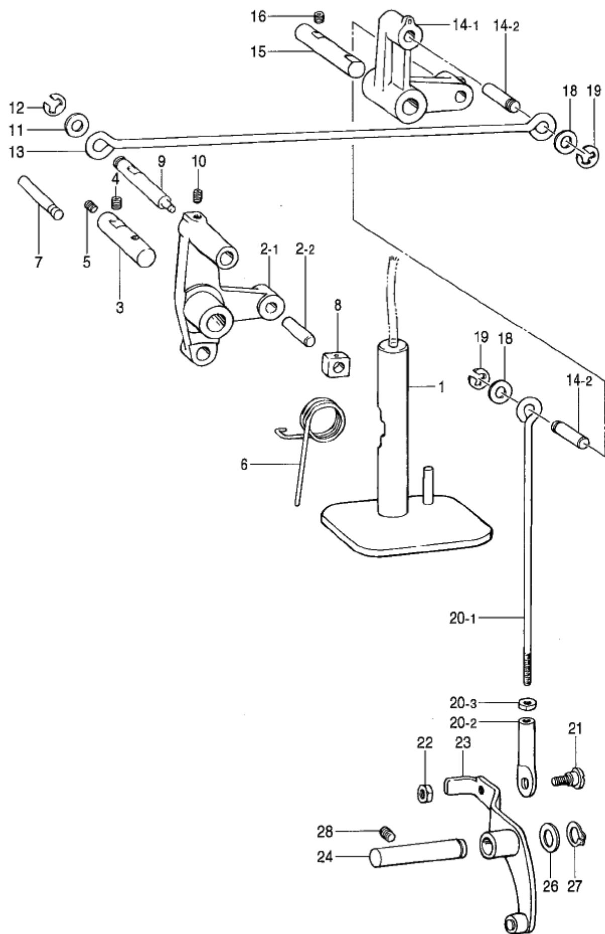
G. 押工上ゲ関係 / Work clamp lifter mechanism
