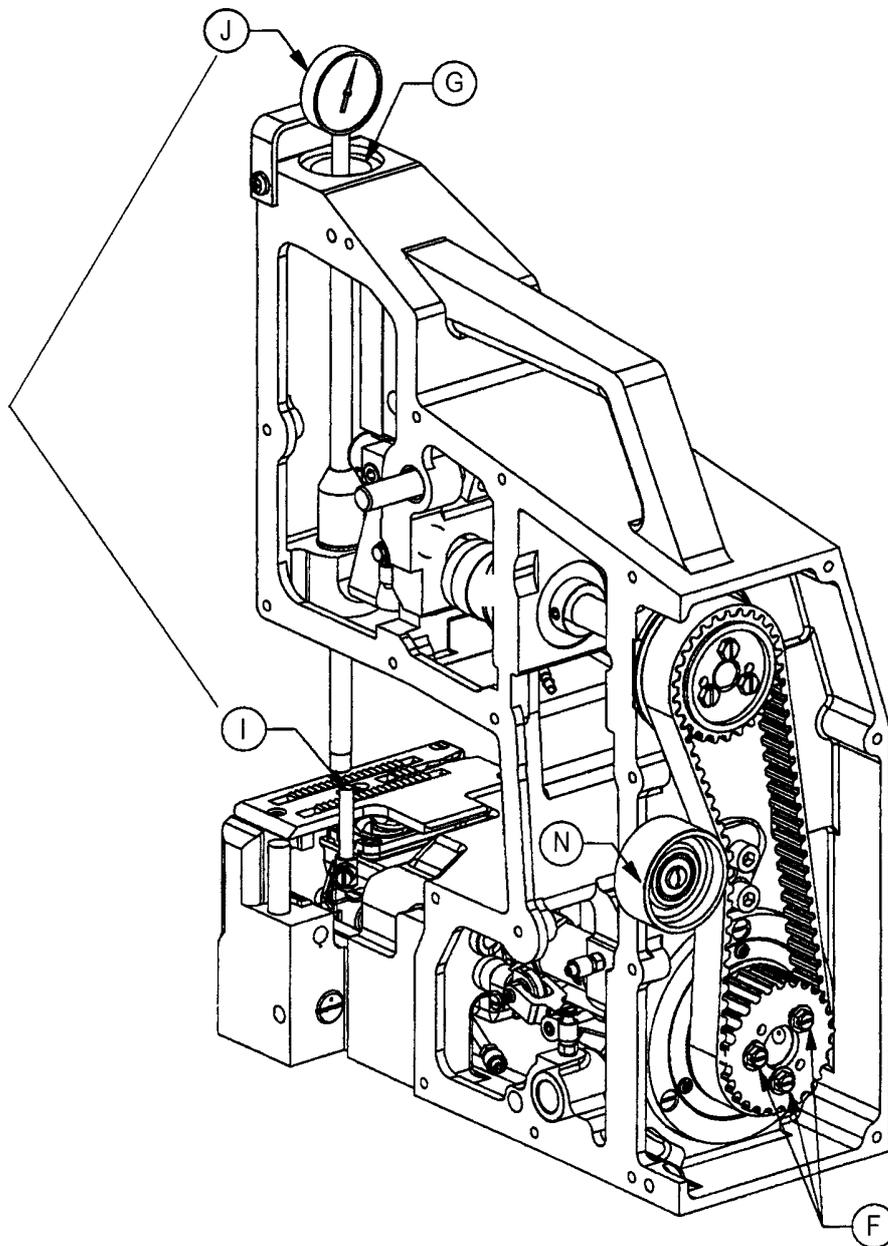
20. Synchronize with TT148 Synchronization Gauge Kit (see **Needle / Looper Synchronisation**).
