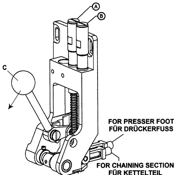
Stop should be set so that when the presser foot is lifted to its maximum position, the foot can not strike the needle head when the needle bar is at bottom dead center.
