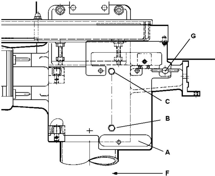
**NOTE:** The base plate A of 20600 Column should be aligned evenly with the two screws B and C and rest with low tension on nut D of eye bolt E. First align sewing head with screw B parallel with feeding direction F. Then thrust screw C against base plate and set nut D with slight clearance to base plate A. Tighten the stops. Secure base plate with Tommy nut G.
