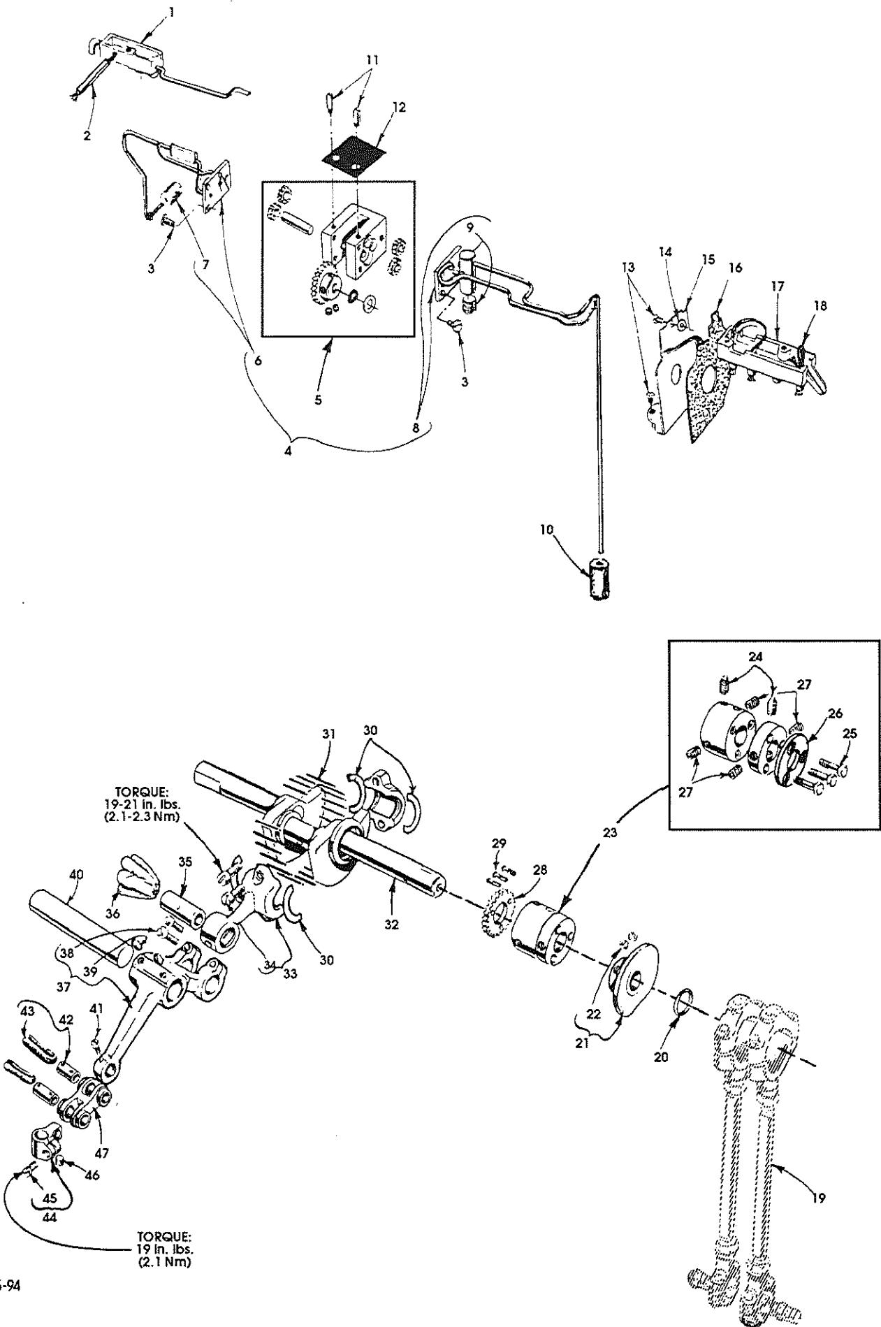
MISCELLANEOUS OILING, NEEDLE LEVER, CRANKSHAFT AND MAIN SHAFT PARTS
