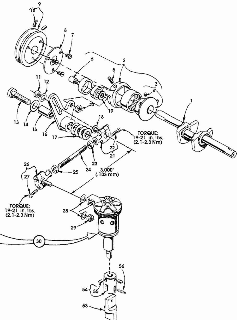
**PULLEY, CRANKSHAFT, CLUTCH AND CLUTCH DRIVING MECHANISM**
