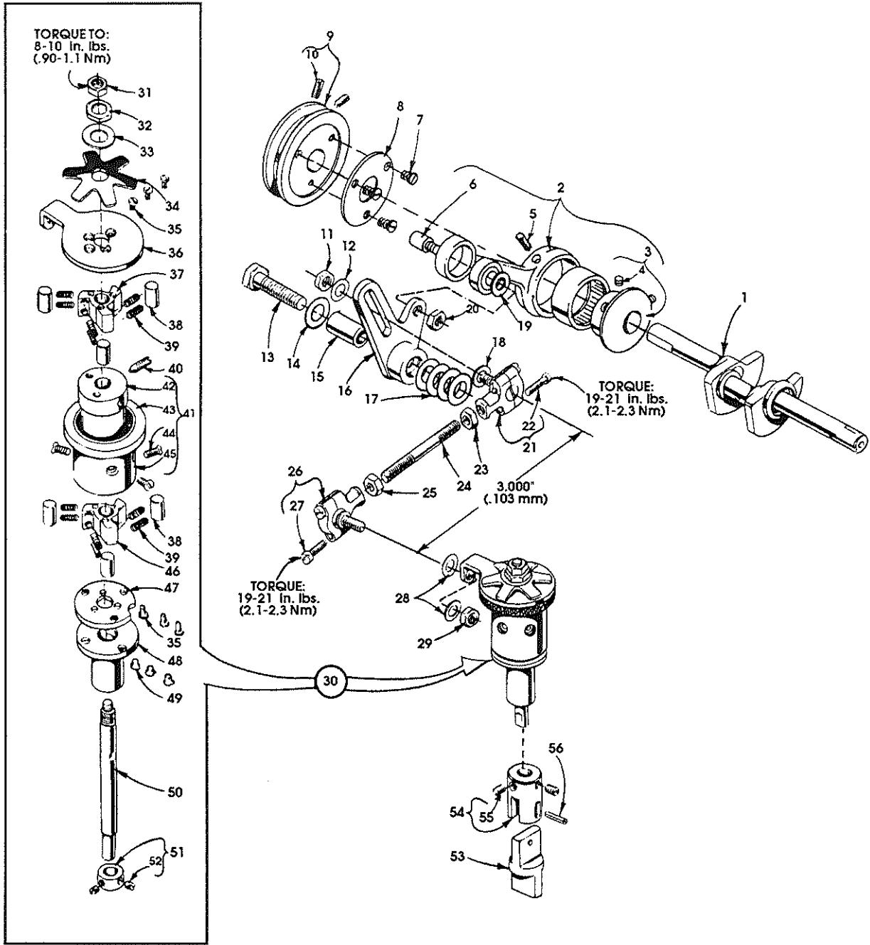
**PULLEY, CRANKSHAFT, CLUTCH AND CLUTCH DRIVING MECHANISM (CONT.)**
