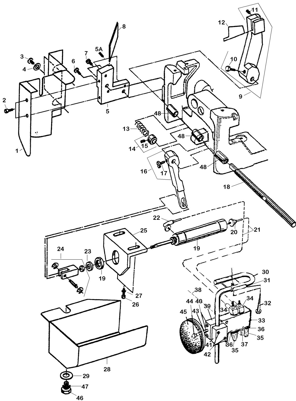
**THREAD CHAIN CUTTER FOR 80700 CD1, PNEUM. DRIVE FROM BELOW**
