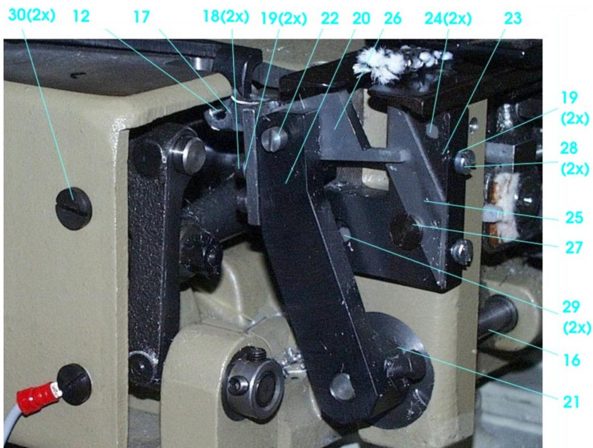
**THREAD CHAIN CUTTER FOR 80700C1, CD1, PNEUM. DRIVE FROM ABOVE**
