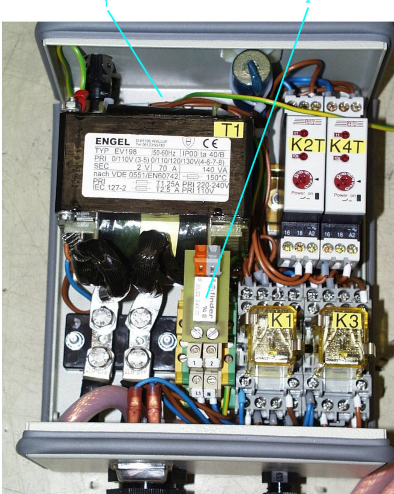
**CONTROL FOR ELECTRO-PNEUMATIC HOT THREAD CHAIN CUTTER 80700C1H, CD1H**
