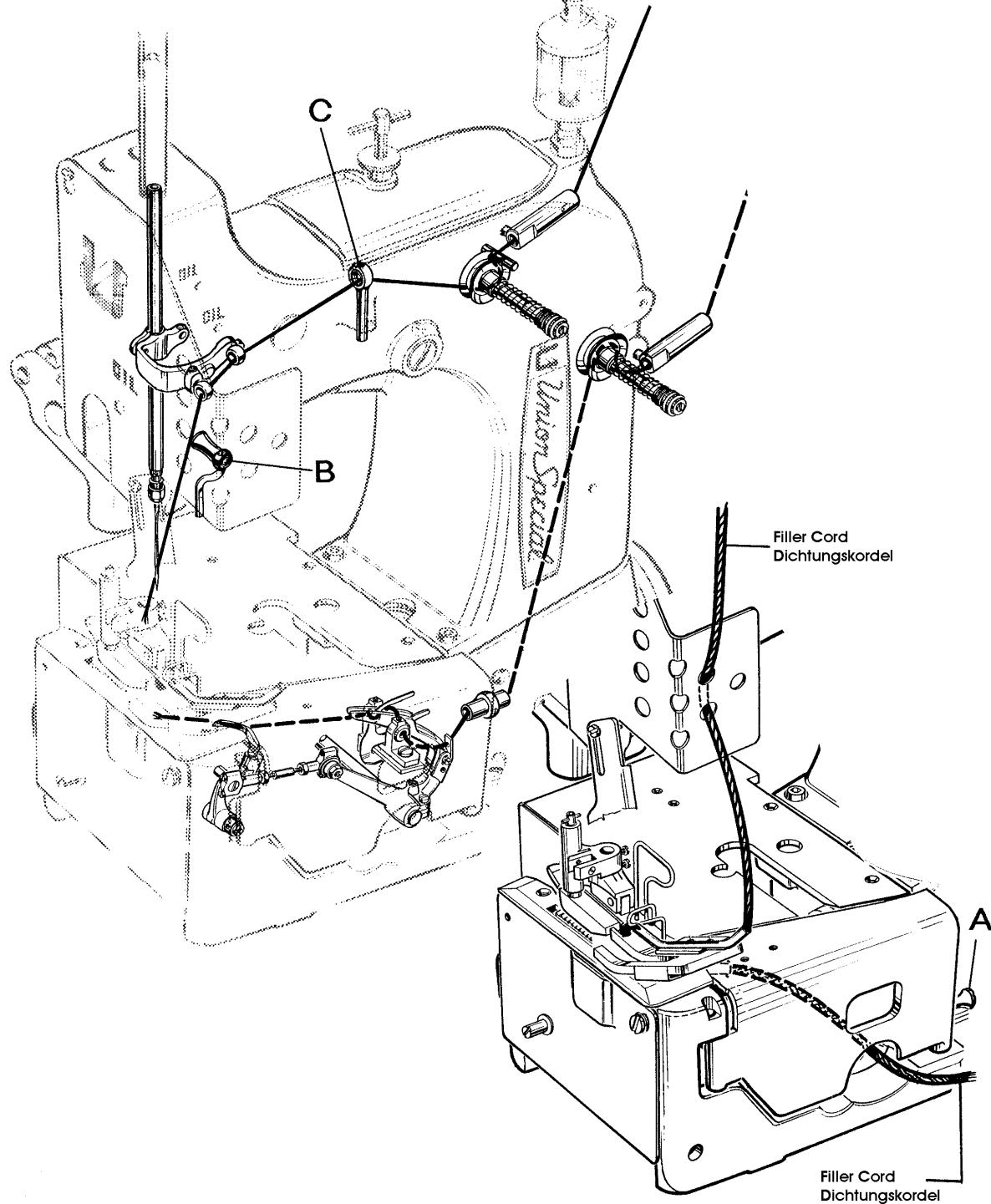
THREADING DIAGRAM FOR STYLES 80700C, C1, C1H, C2
