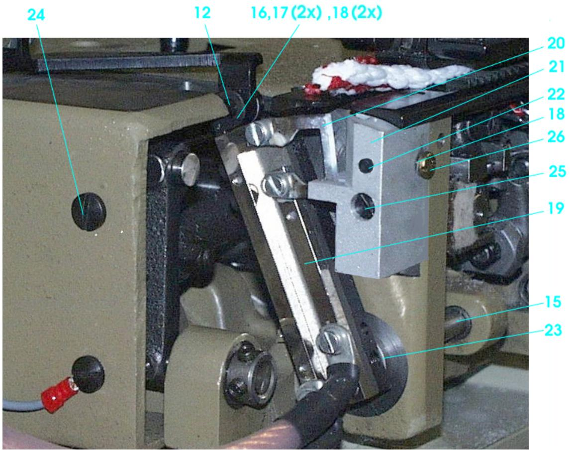
**HOT THREAD CHAIN CUTTER FOR 80700C1H, CD1H**
