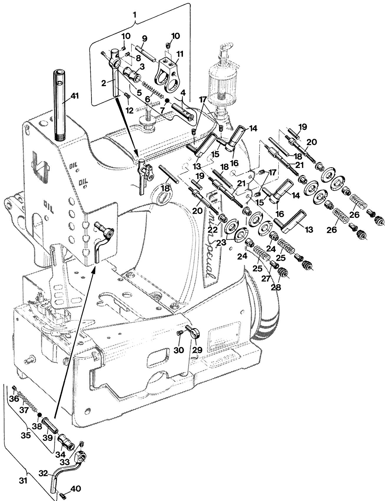
**THREAD TENSIONS, THREAD GUIDES AND NEEDLE BAR GUARD FOR 80700CD, CD1, CD1H, CD2**
