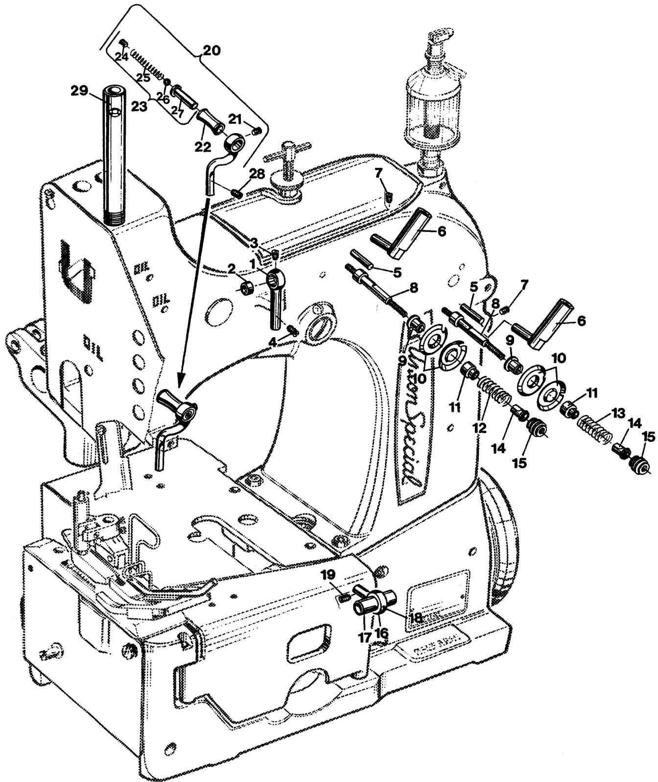
**THREAD TENSION, THREAD GUIDES AND NEEDLE BAR GUARD FOR 80700C, C1, C1H, C2**
