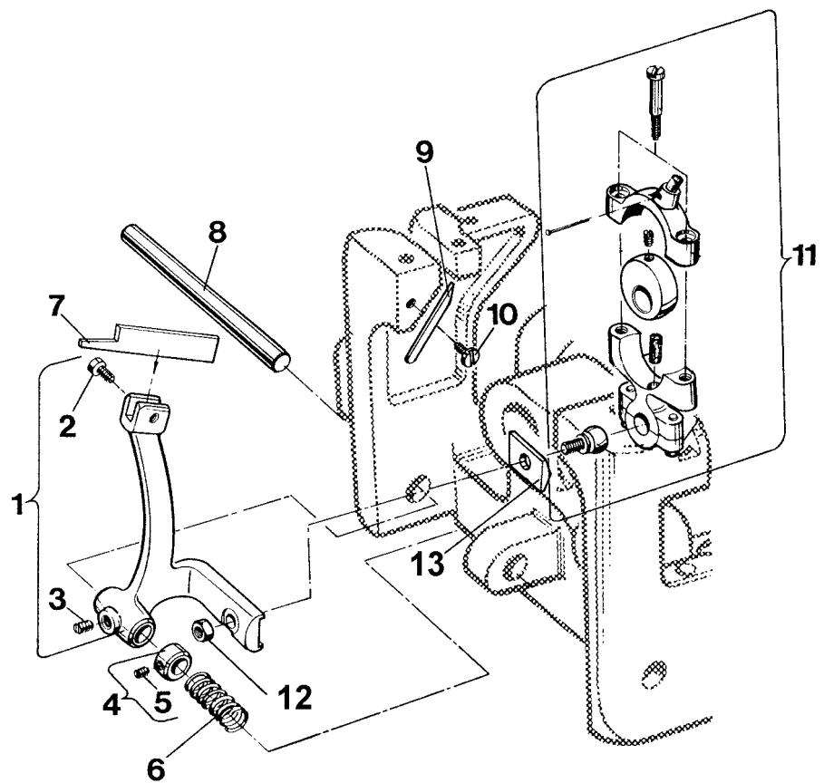
**THREAD CHAIN CUTTER KNIVES AND CHAIN CUTTER DRIVE FOR 80700 C, CD**
