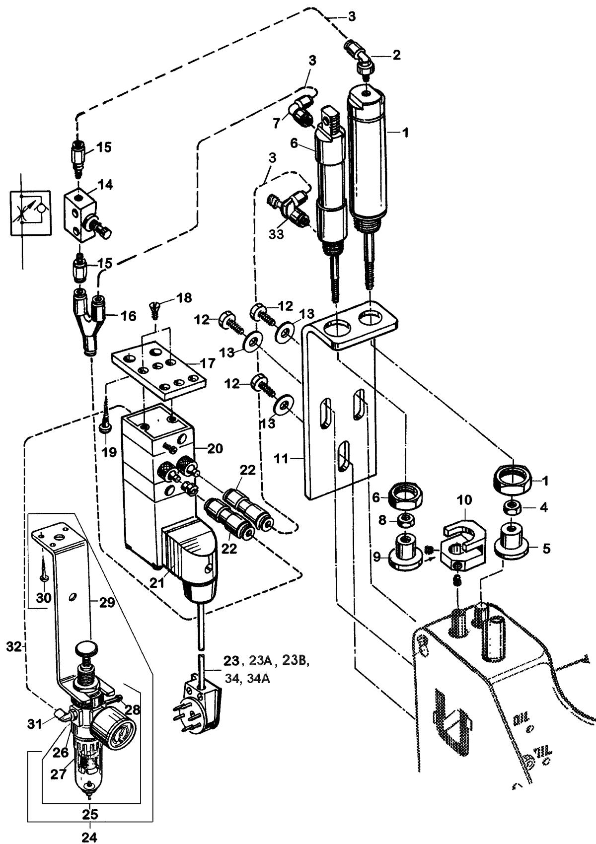
**ELECTRO-PNEUMATIC PARTS KIT FOR UPPER FEED PRESSURE AND LIFTER FOR 80700 WITH ELECTRONIC DRIVE**
