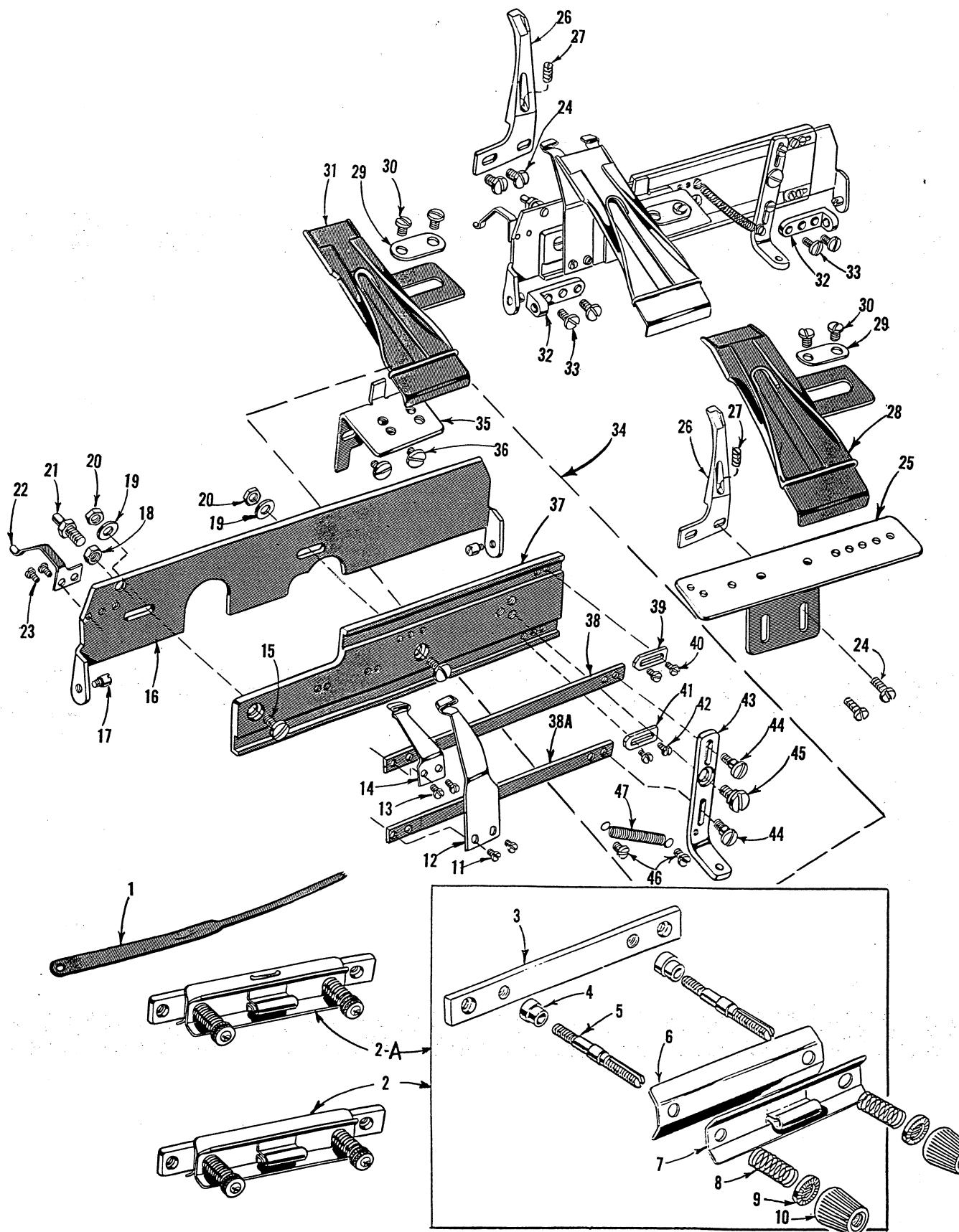
ATTACHMENTS, STRIP TENSIONS AND COLLAPSING MECHANISM
