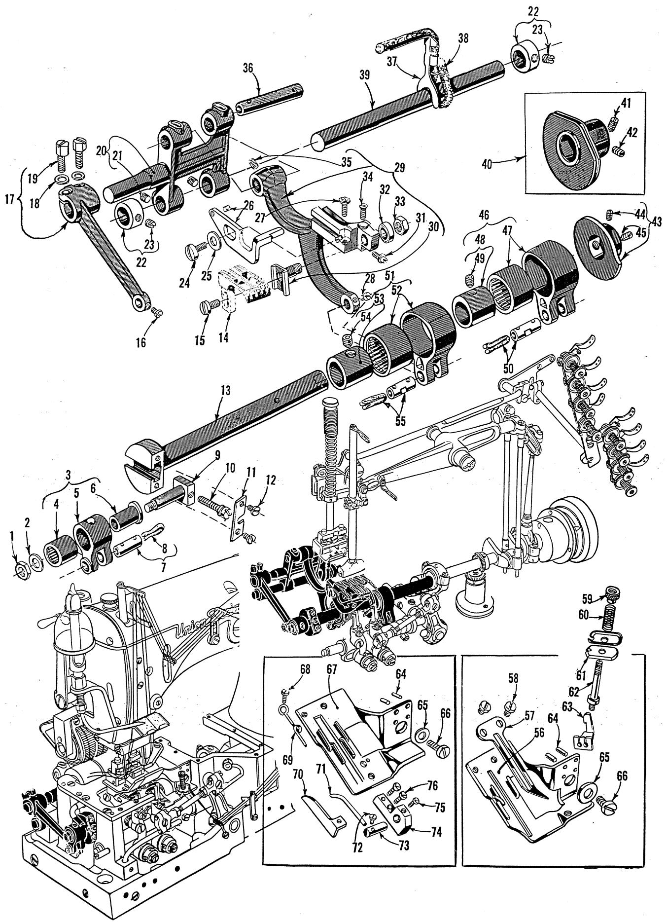
MAIN SHAFT, FEED DRIVING PARTS AND LOOPER THREAD TAKE-UP PARTS
