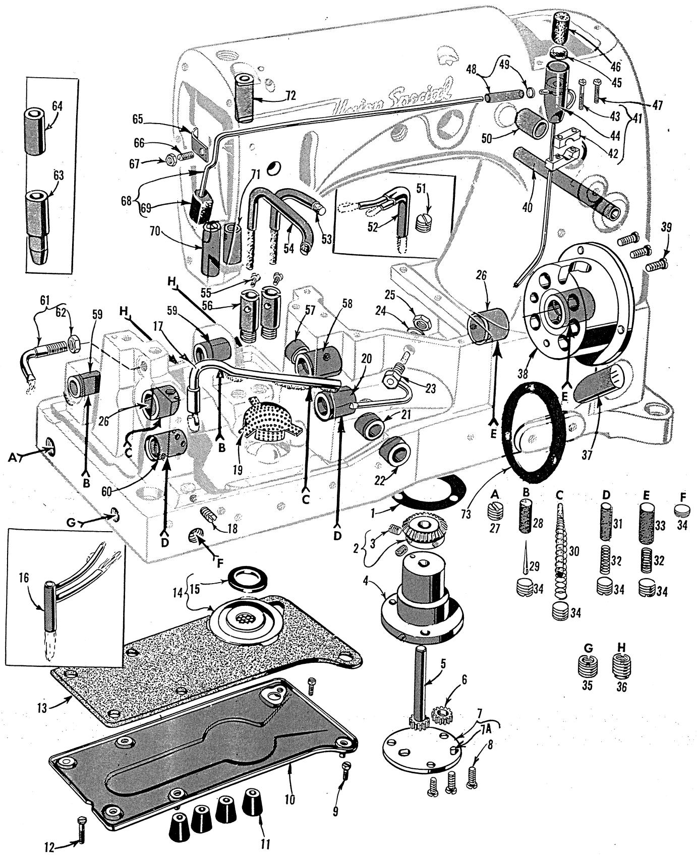
MAIN FRAME, BUSHINGS AND MISCELLANEOUS OILING PARTS
