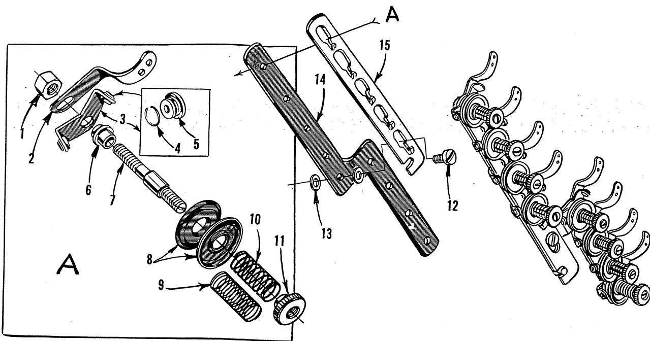
THREAD TENSION AND LIFTER LEVER PARTS
