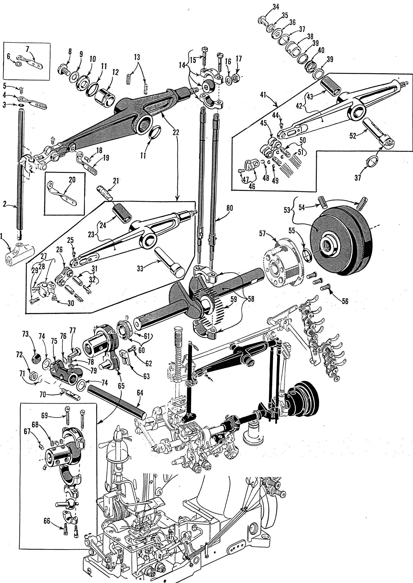
CRANKSHAFT, NEEDLE LEVER AND LOOPER DRIVING PARTS
