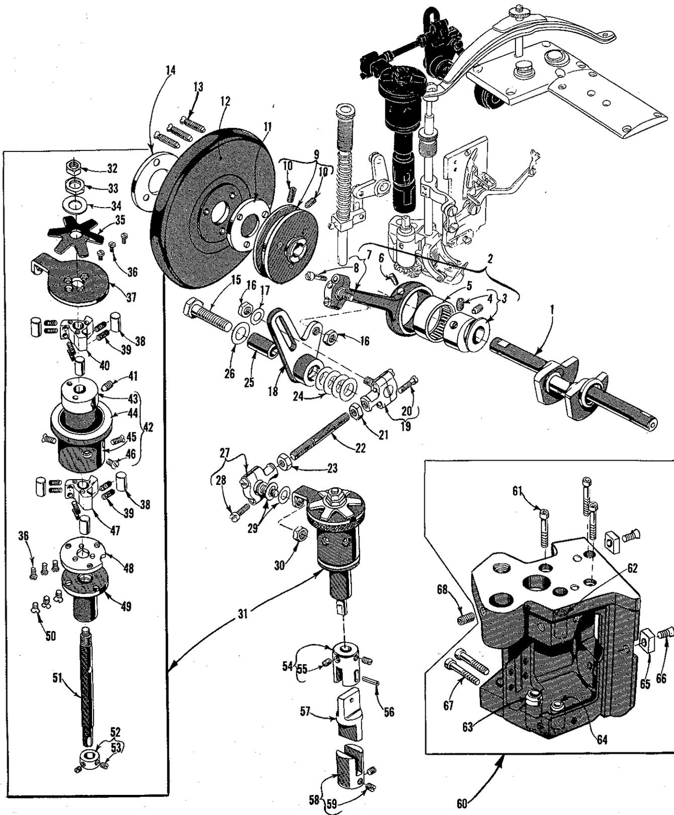
PULLEY, CRANKSHAFT, CLUTCH AND CLUTCH DRIVING MECHANISM
