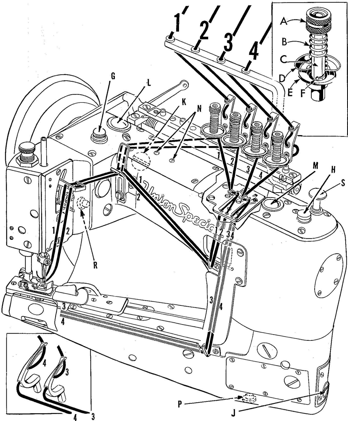
OILING AND THREADING DIAGRAM FOR ALL STYLES IN CLASS 35700, EXCEPT STYLES 35700 BS AND DS.
