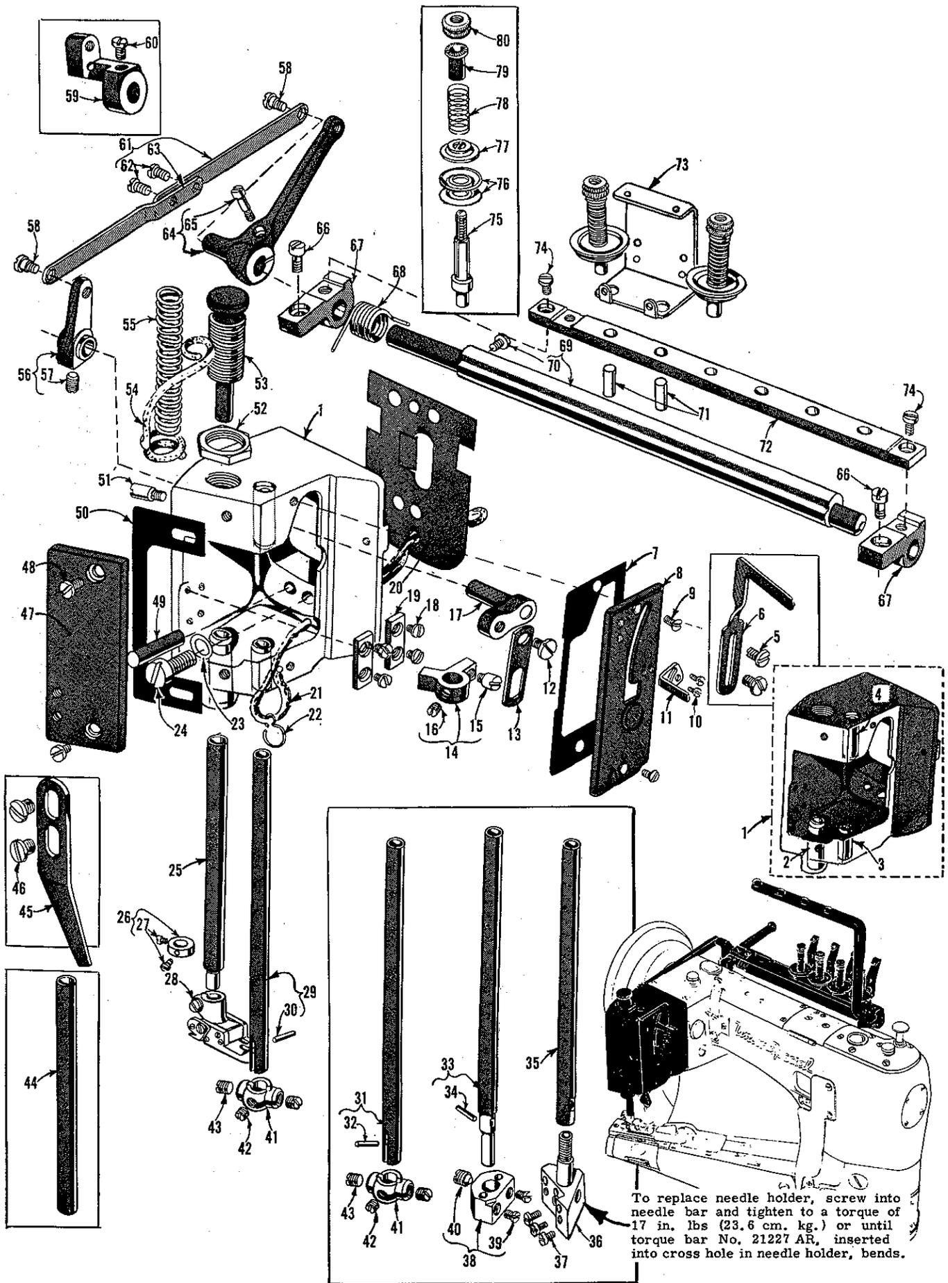
To replace needle holder, screw into needle bar and tighten to a torque of 17 in. lbs (23.6 cm. kg.) or until torque bar No. 21227 AR, inserted into cross hole in needle holder, bends.
