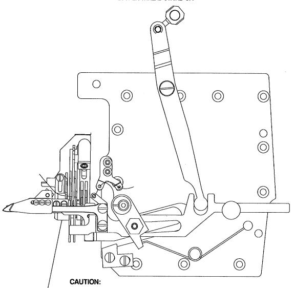
IMPROPER THREADING MAY CAUSE; LOOPER THREAD WRAP-UPS OR INCONSISTENT START OF STITCHES
