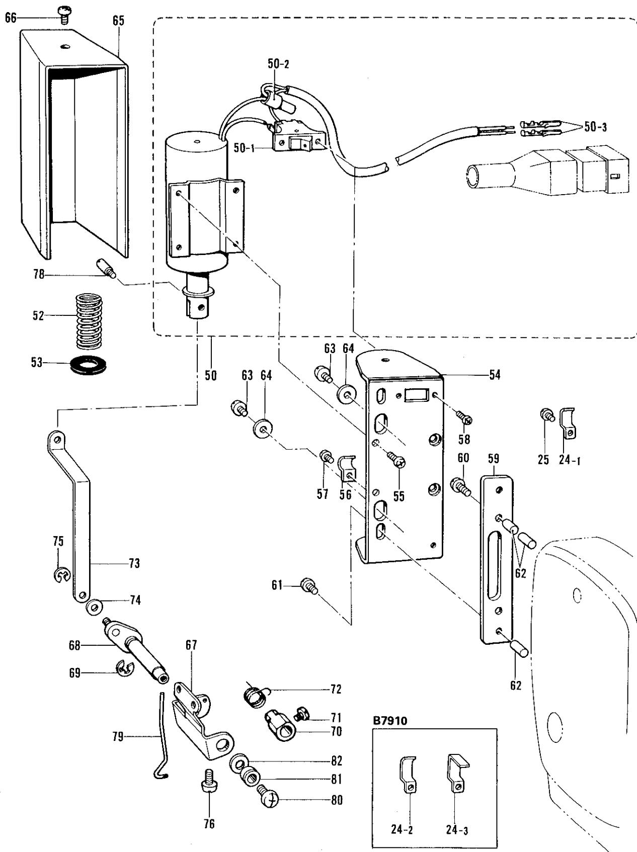
P. 糸扱い関係 / Thread wiper mechanism / Fadenspannvorrichtung /
