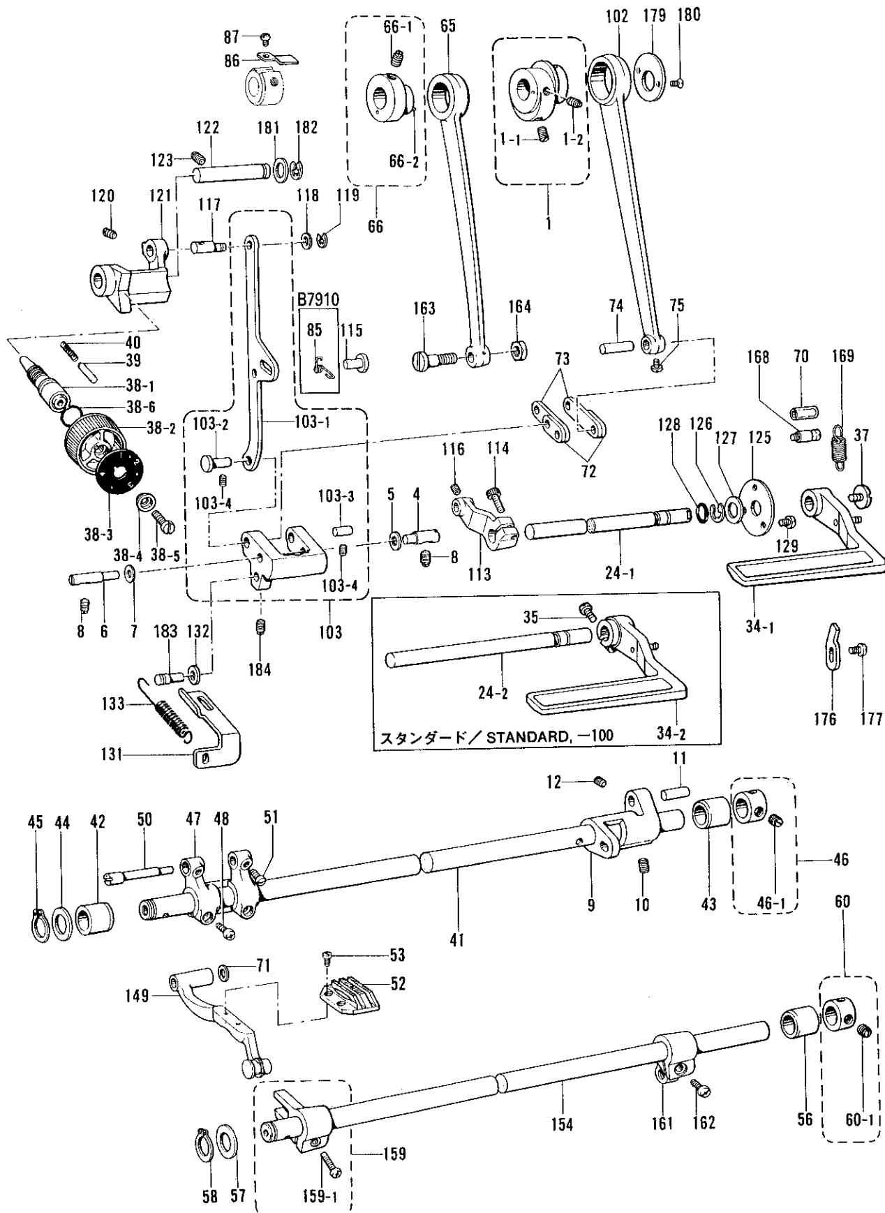
F. 送り関係 / Feed mechanism / Transportvorrichtung /
