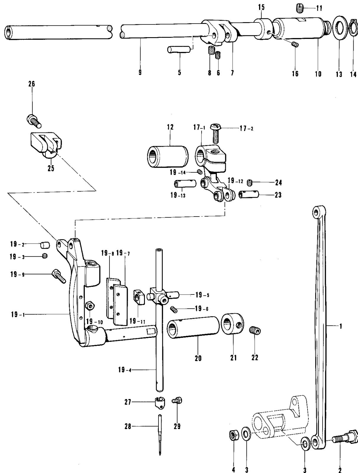
D. 針送り関係 / Needle feed mechanism / Nadelstange transport vorrichtung /
