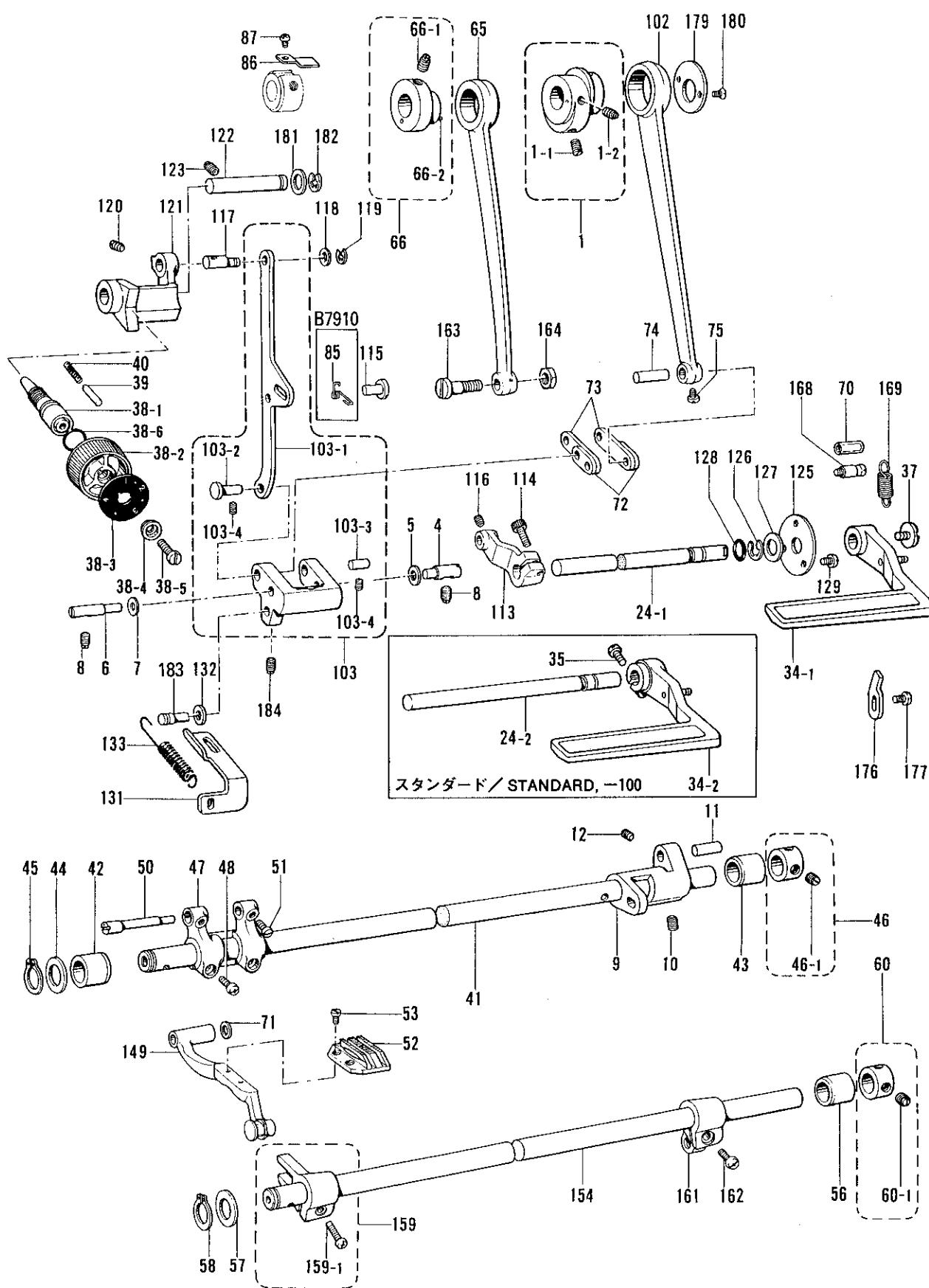
F. 送り関係 / Feed mechanism / Transportvorrichtung /
