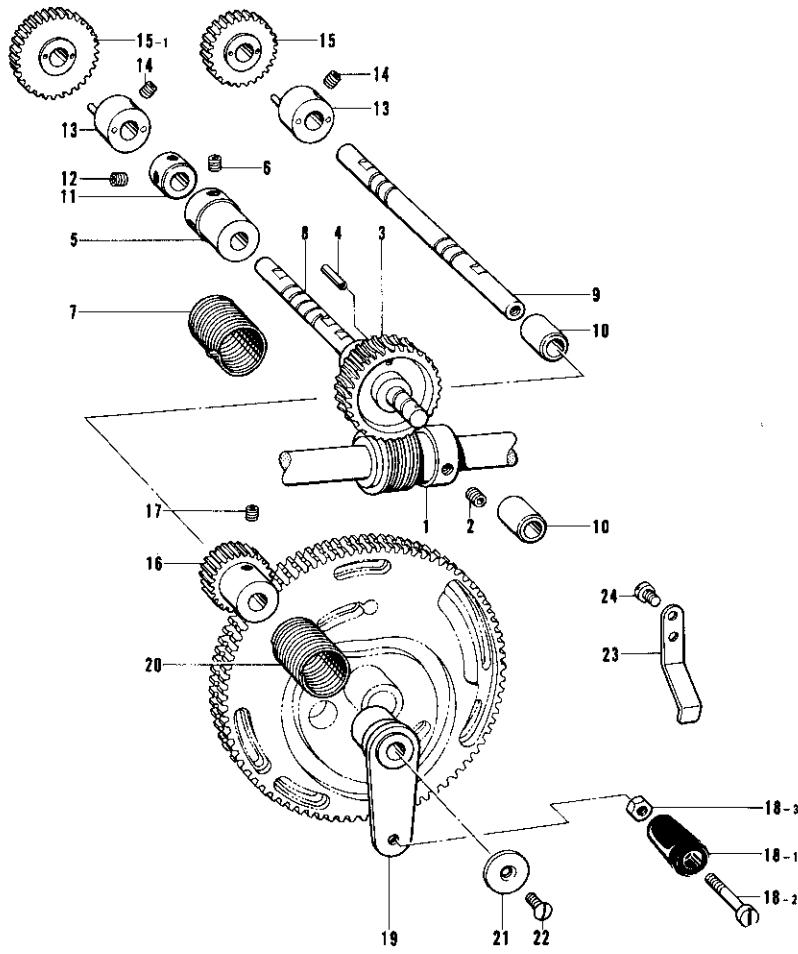
**N. Thread breakage detector**
