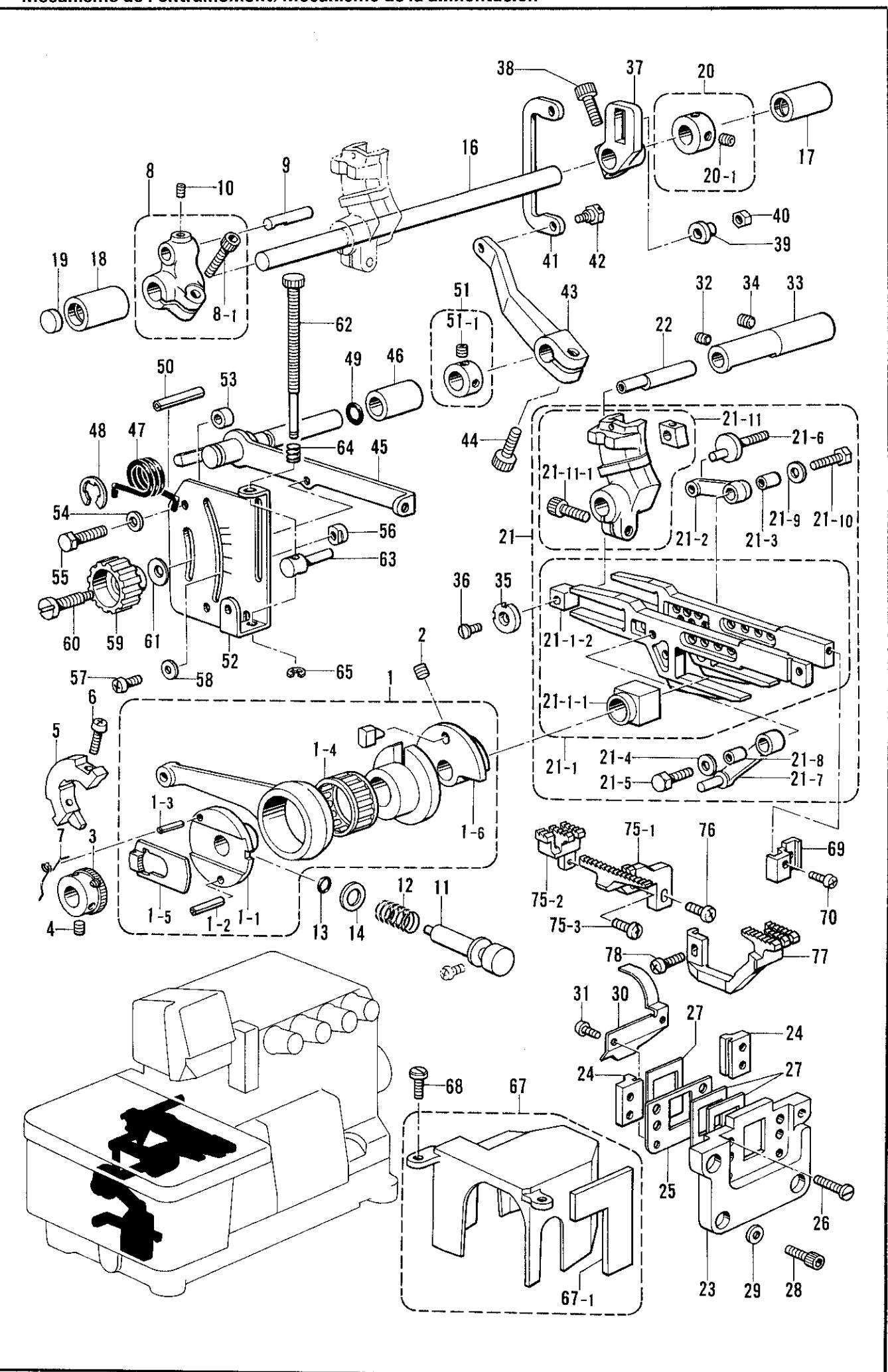
E. 送り関係/Feed mechanism/Transportvorrichtung/
