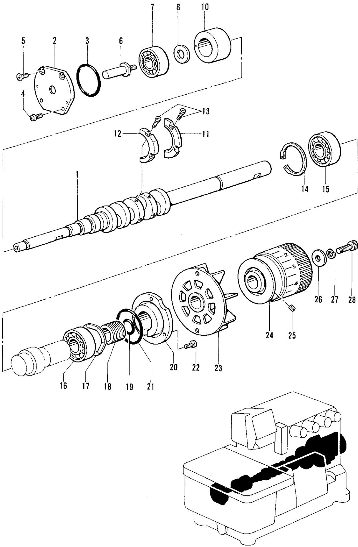
B. 駆動軸関係/Crank shaft mechanism/Kurbelwelle/
