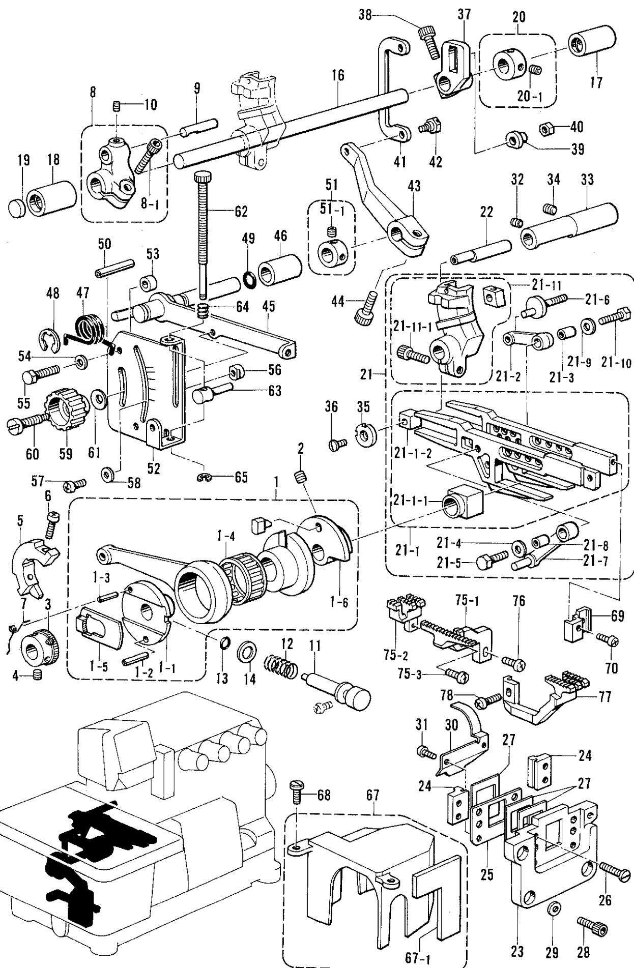
E. 送り関係/Feed mechanism/Transportvorrichtung/
