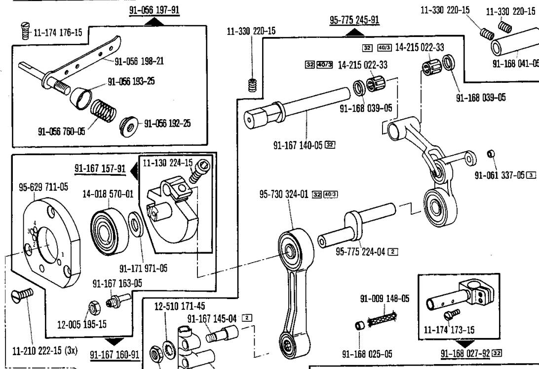
Part number 91-167 160-91 is for a needle bar stroke of 37mm. □
