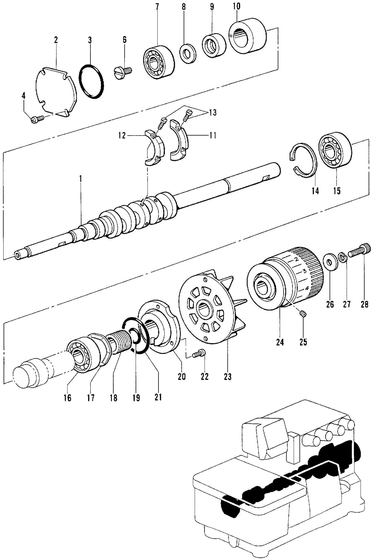
B. 駆動軸関係/Crank shaft mechanism/Kurbelwelle/
