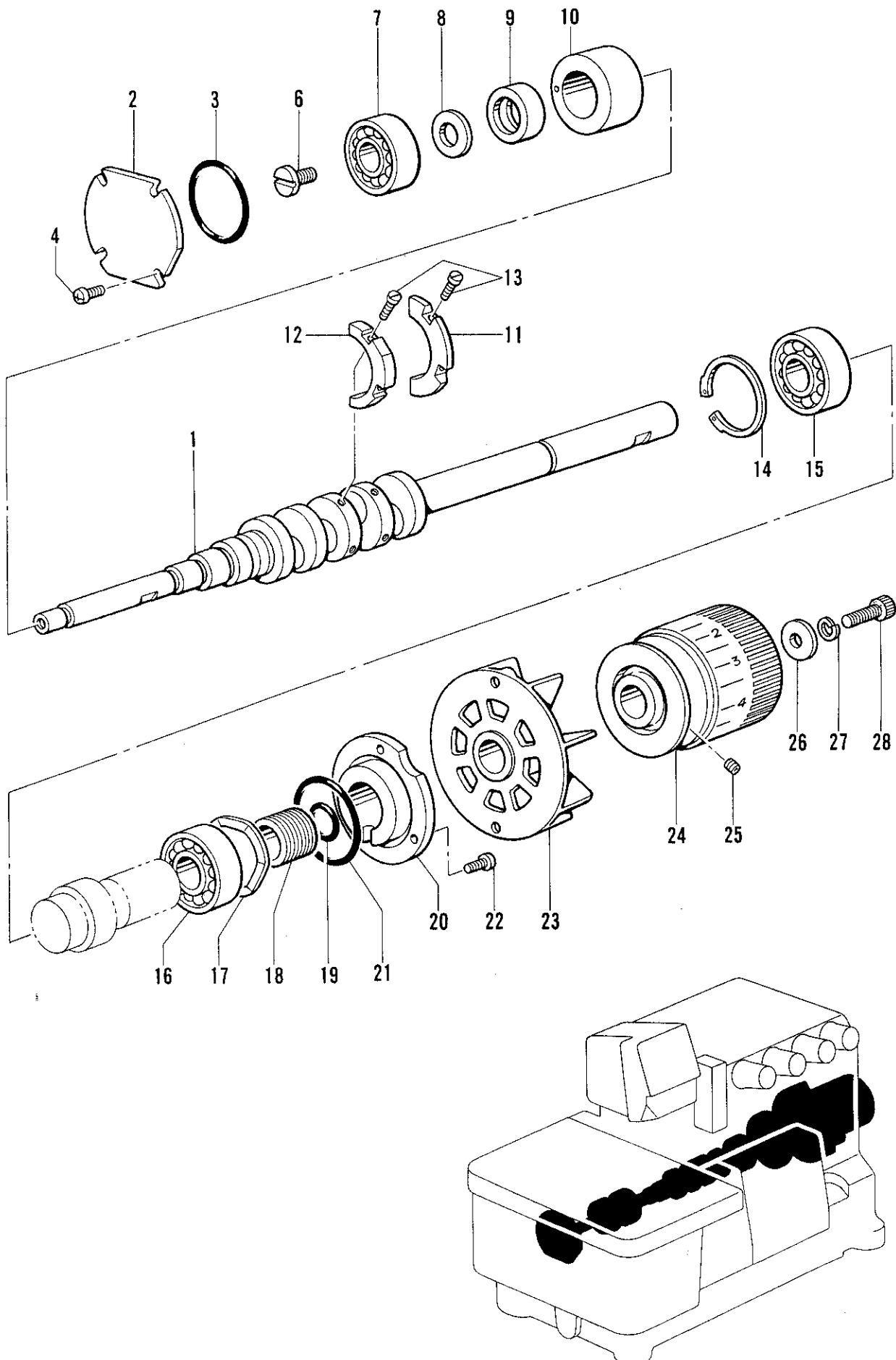
B. 駆動軸関係/Crank shaft mechanism/Kurbelwelle/
