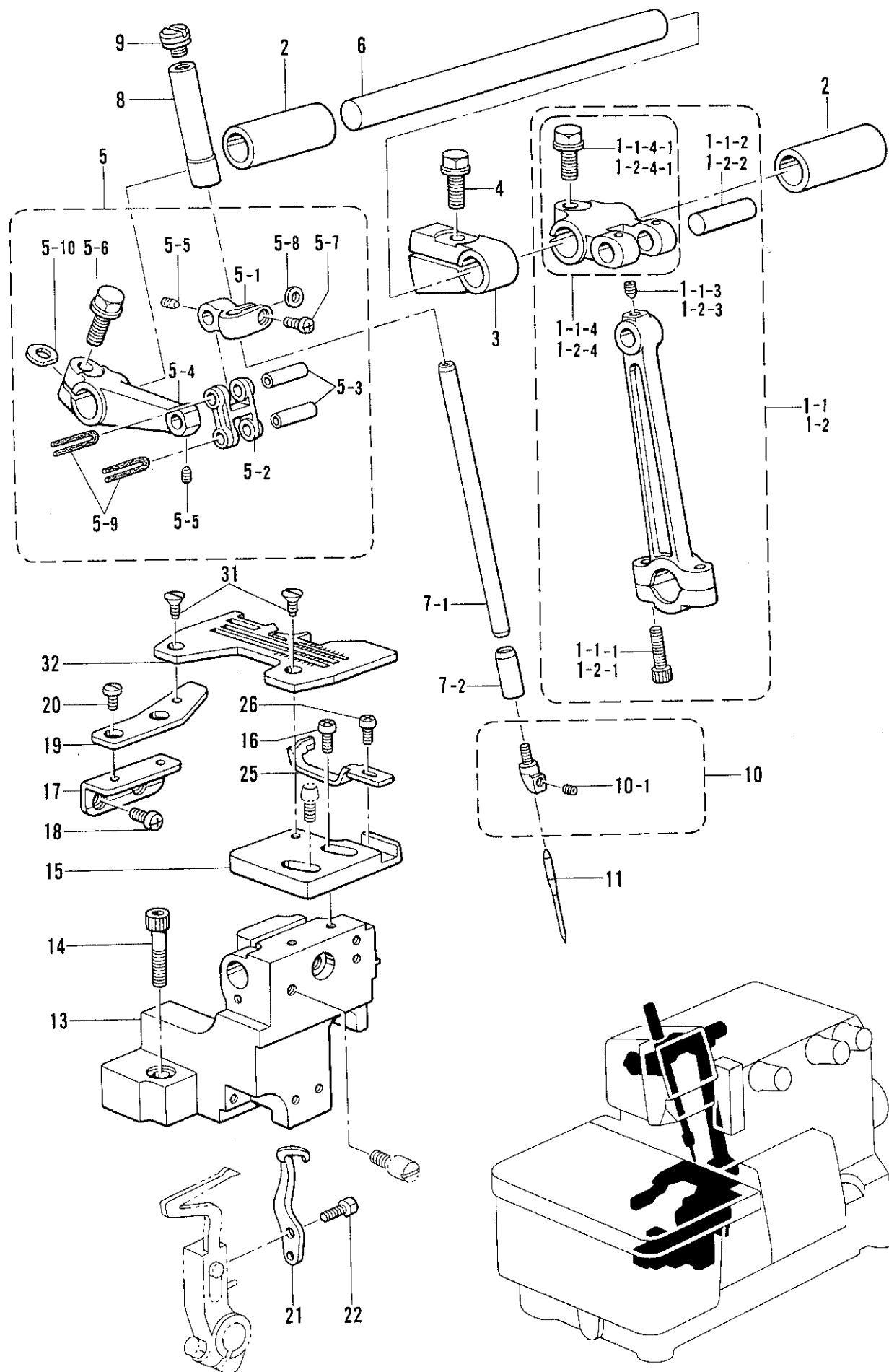
C. 針棒関係 /Needle bar mechanism/Nadelstangenvorrichtung/
