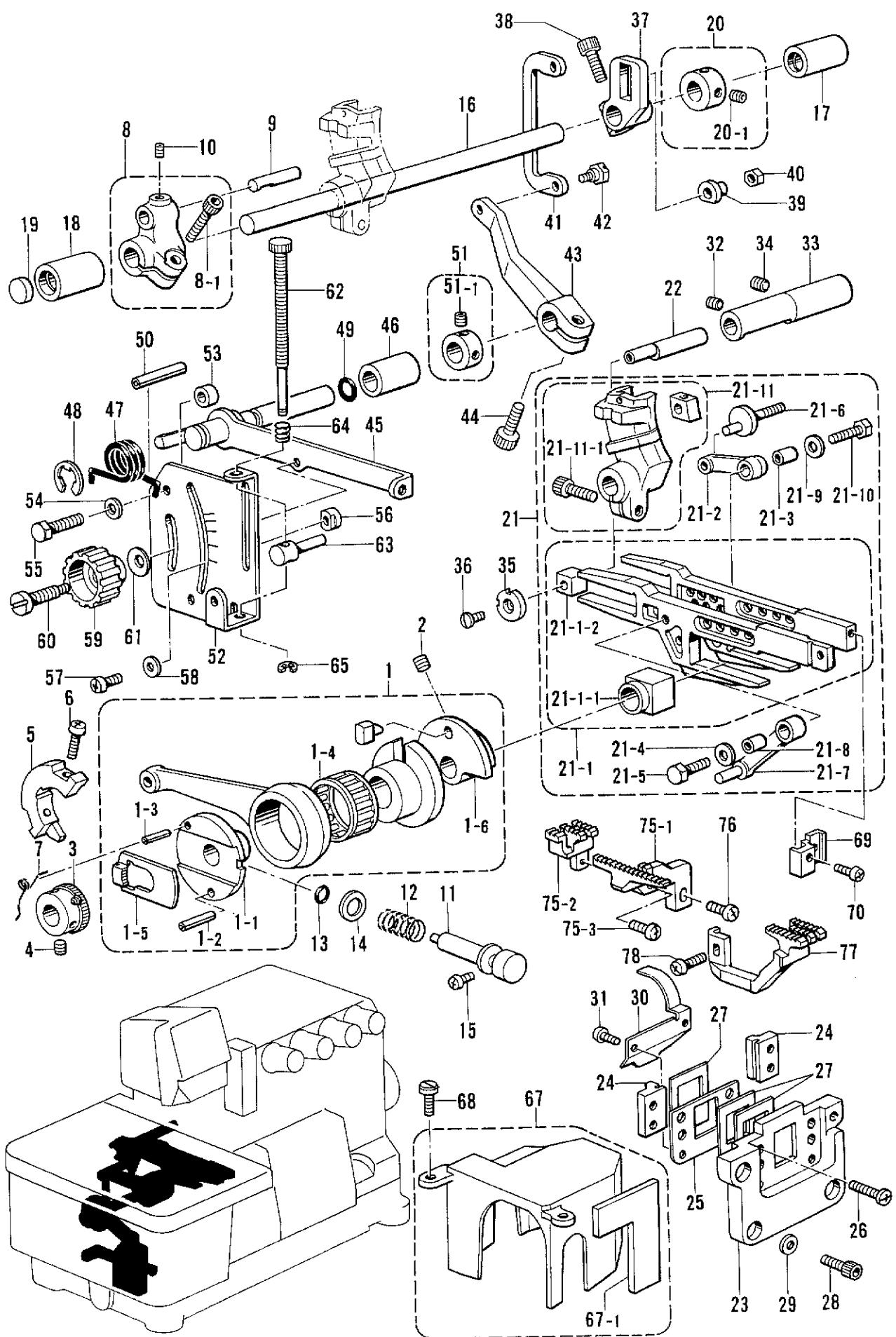
E. 送り関係/Feed mechanism/Transportvorrichtung/
