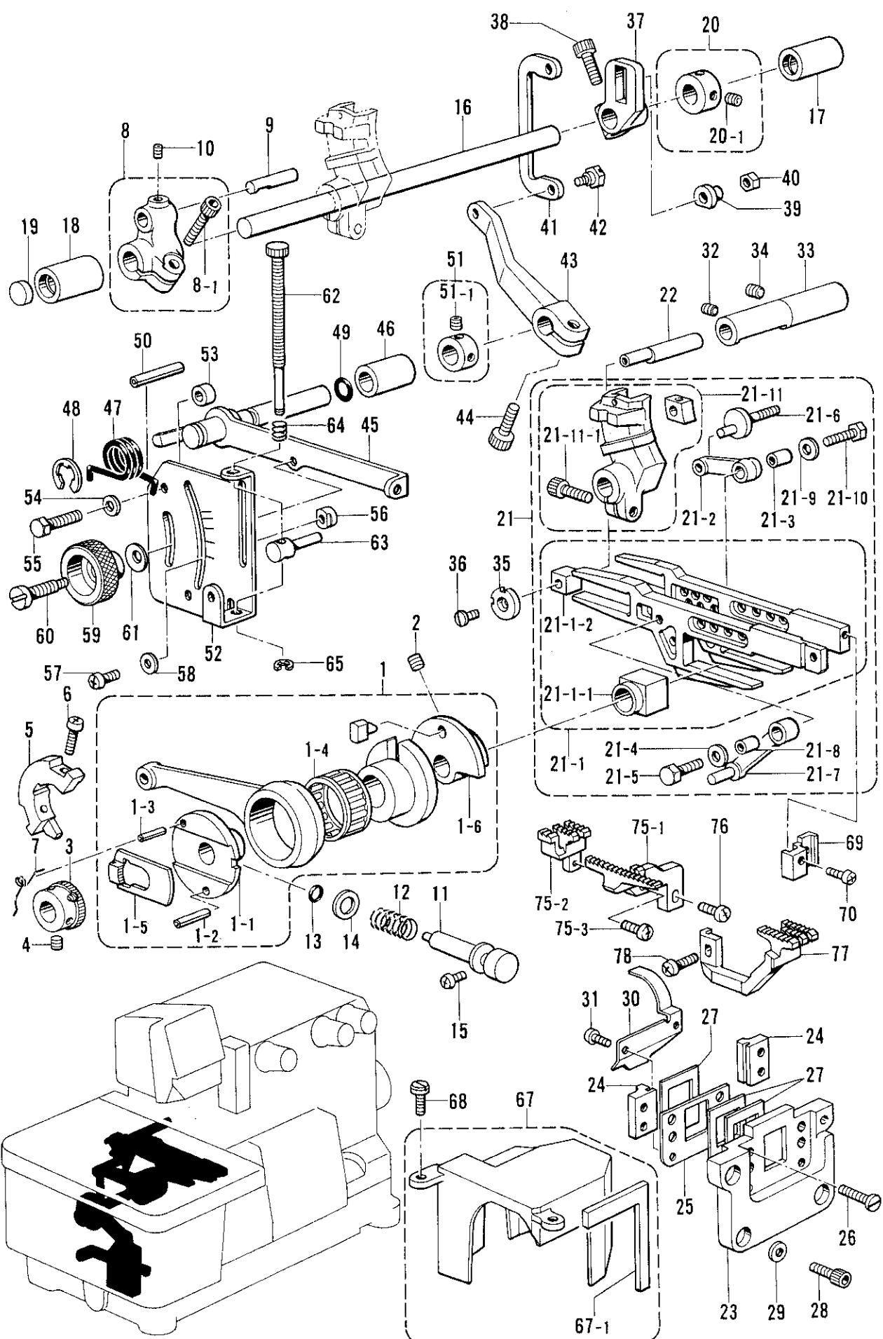
E. 送り関係 /Feed mechanism/Transportvorrichtung/
