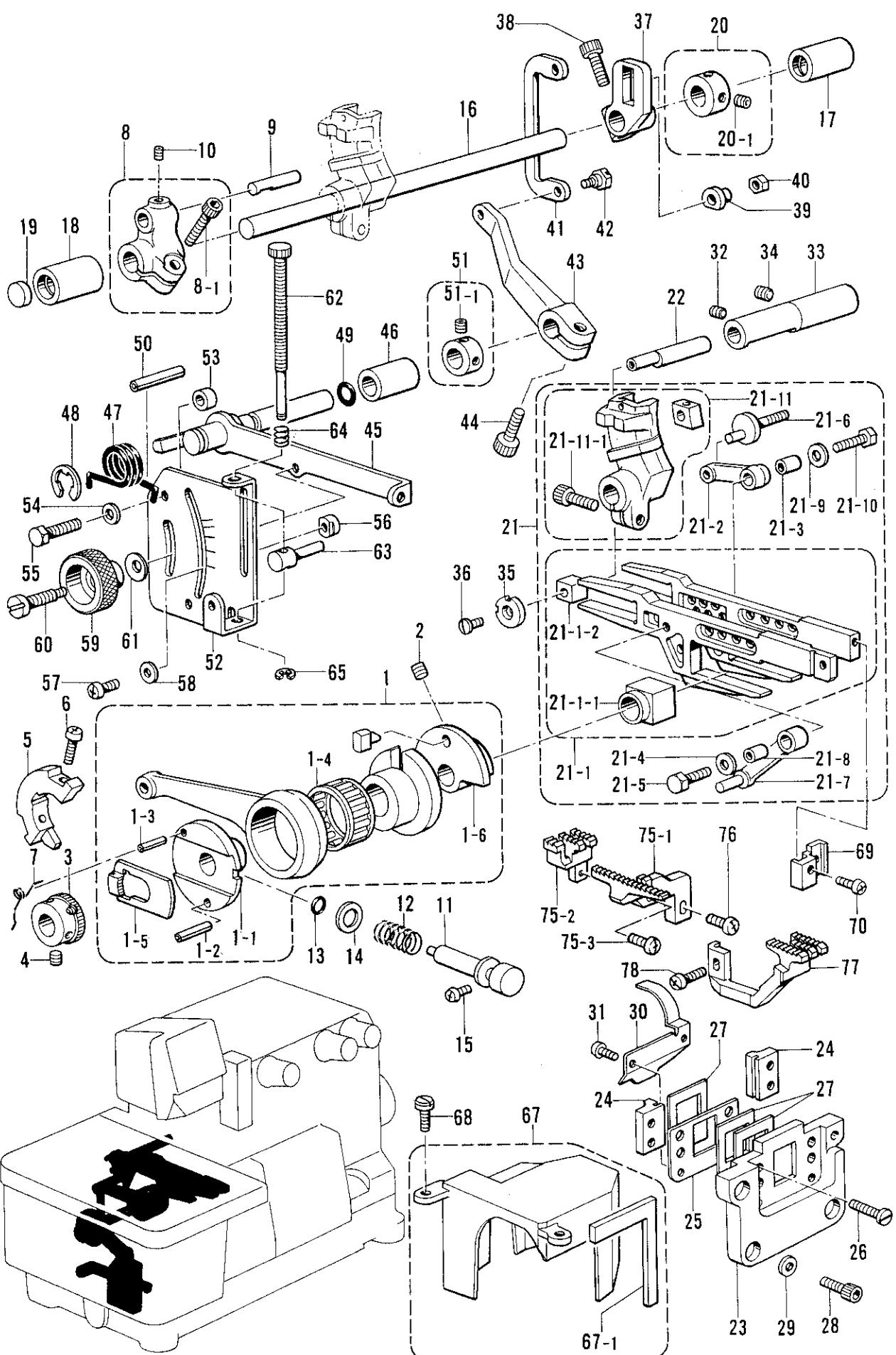
E. 送り関係/Feed mechanism/Transportvorrichtung/
