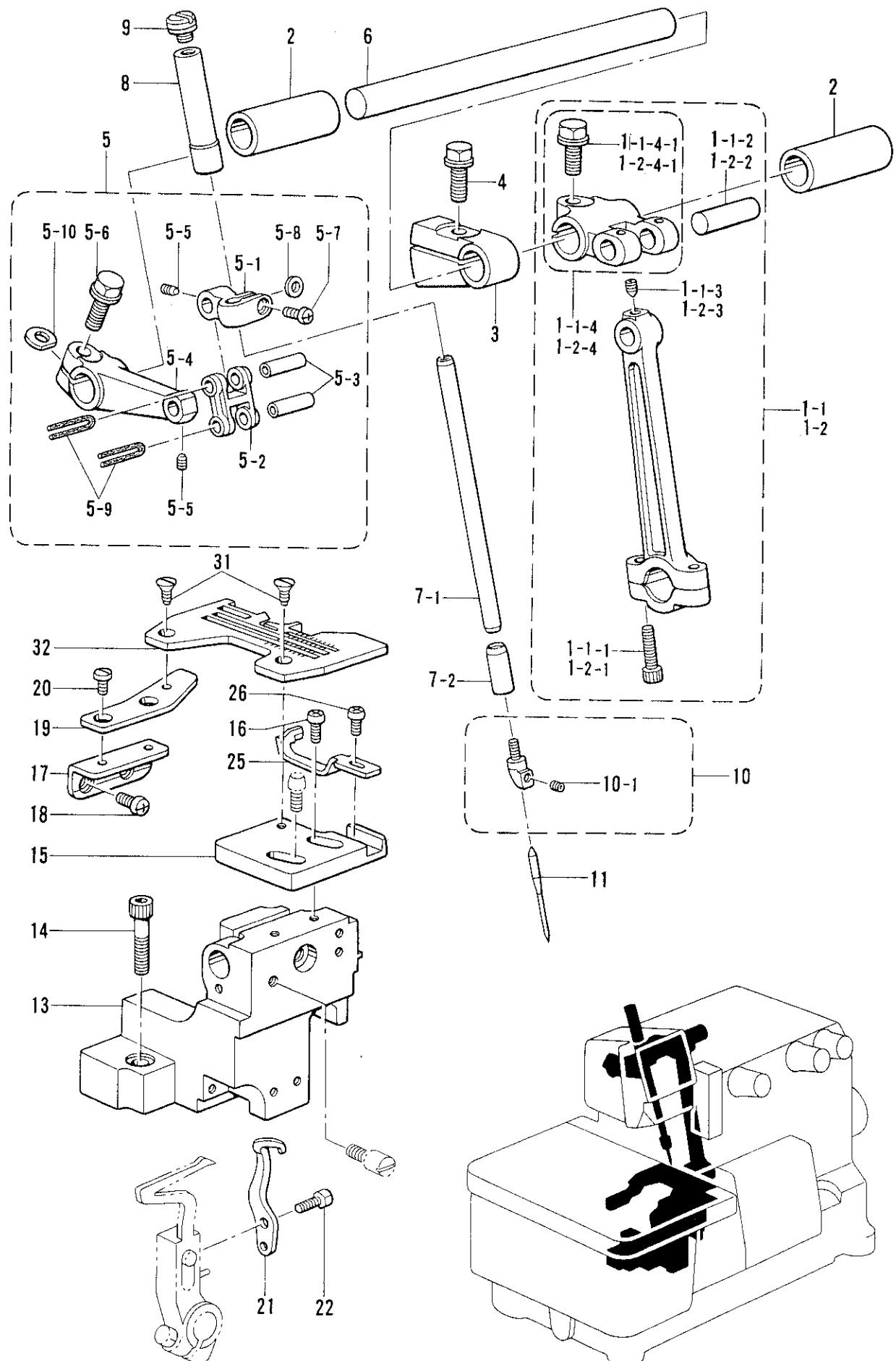
C. 針棒関係 /Needle bar mechanism/Nadelstangenvorrichtung/
