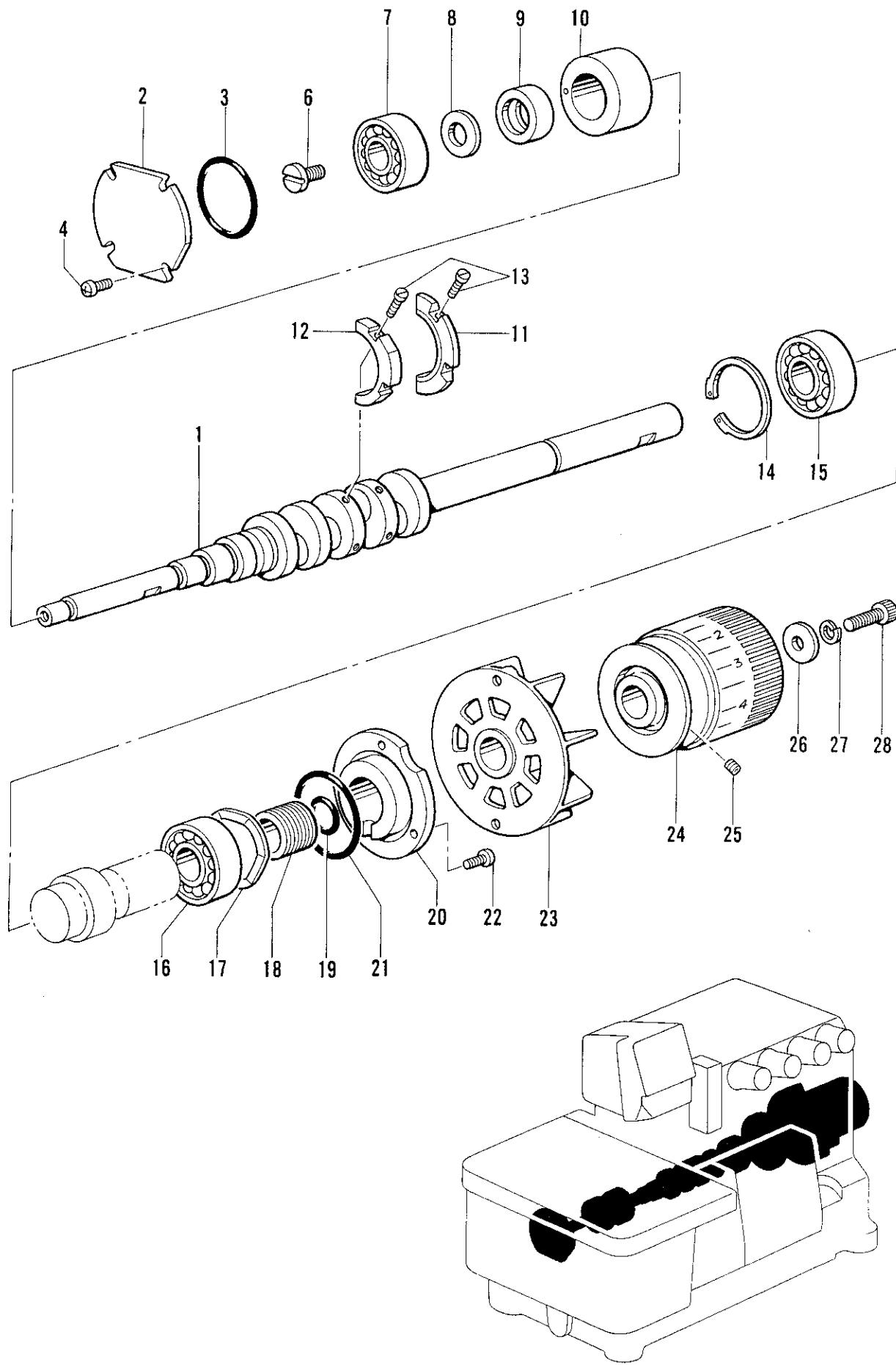
B. 駆動軸関係/Crank shaft mechanism/Kurbelwelle/
