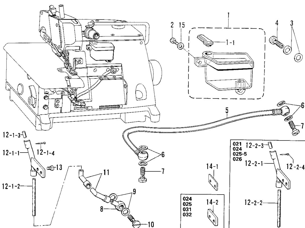
B. 駆動軸関係/Crank shaft mechanism /Kurbelwelle/
