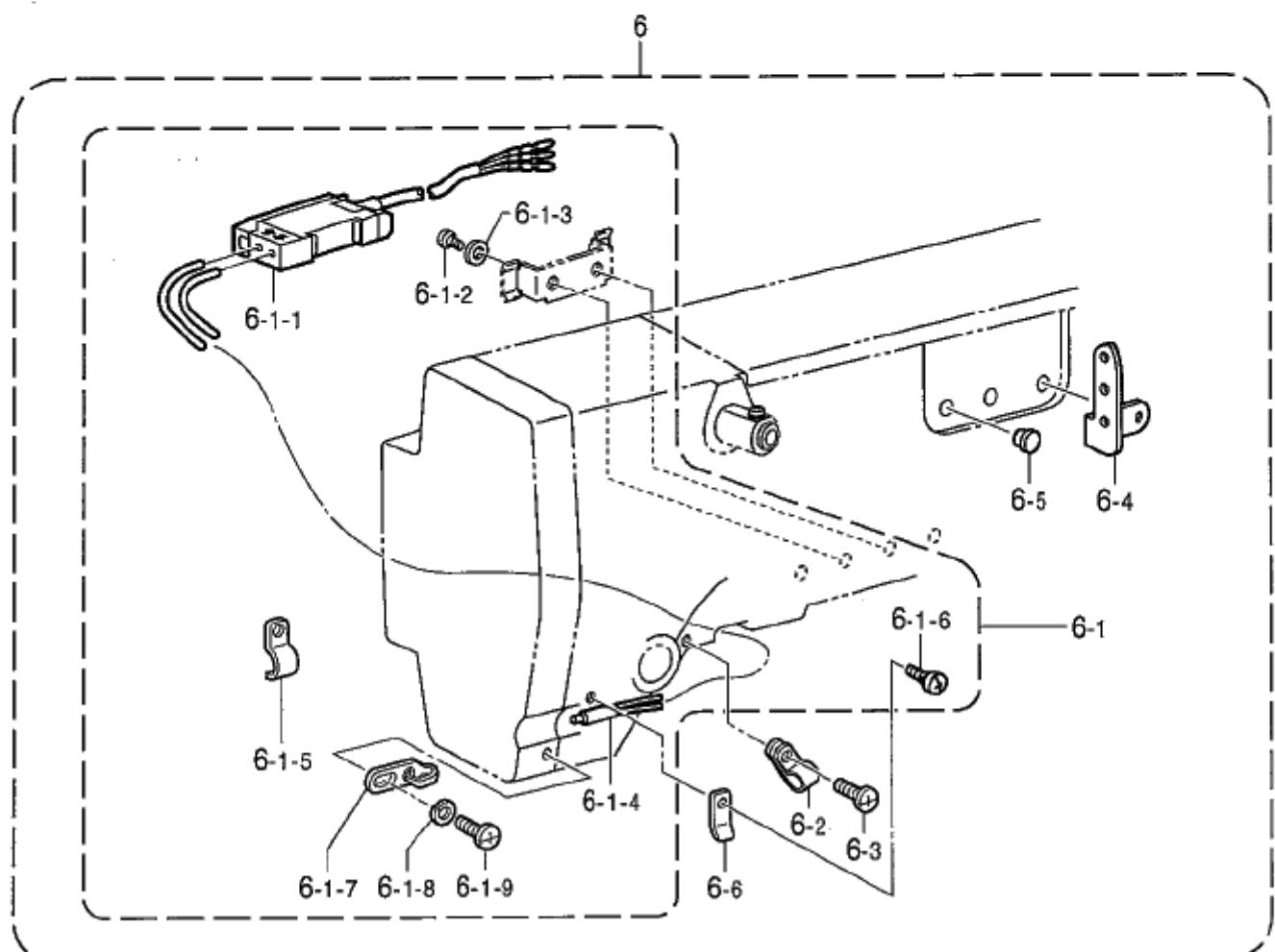
E. 糸切レ感知関係 / Thread breakage detector mechanism
