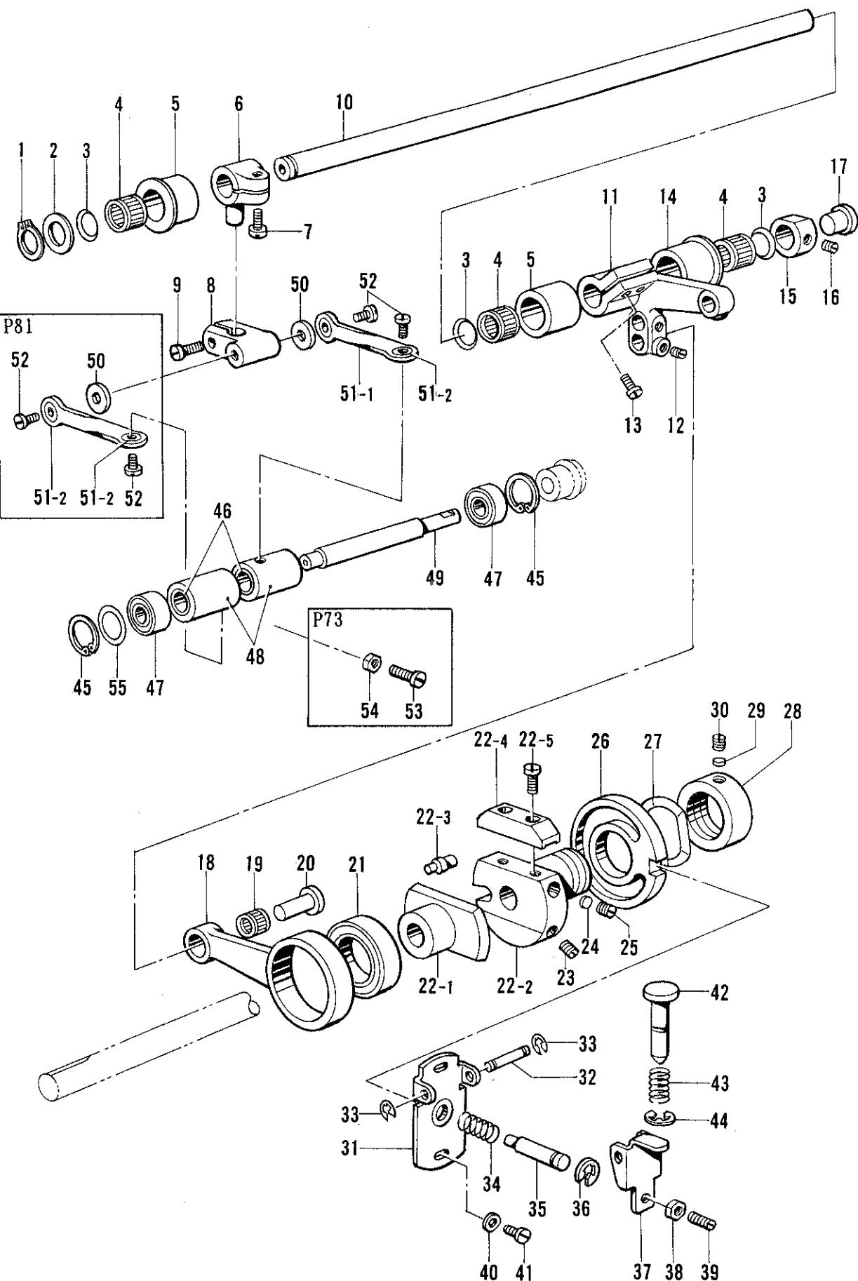
D. 送り関係/Feed mechanism/Transportvorrichtung/
