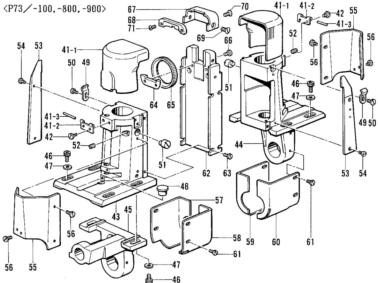
J5. カマ関係/Rotary hook mechanism/Greifervorrichtung/
