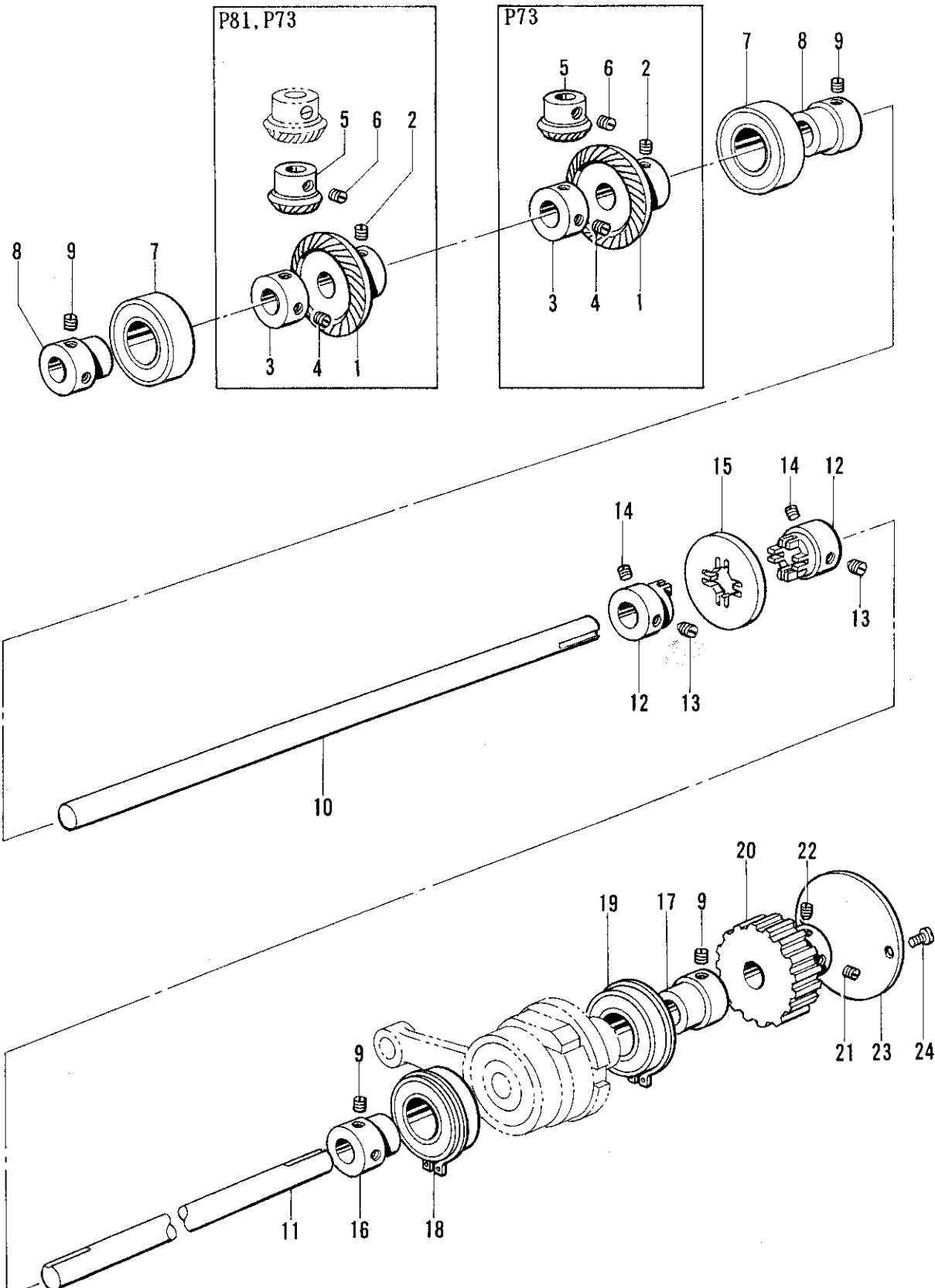
H. 下軸関係/Lower shaft mechanism/Untere Welle/
