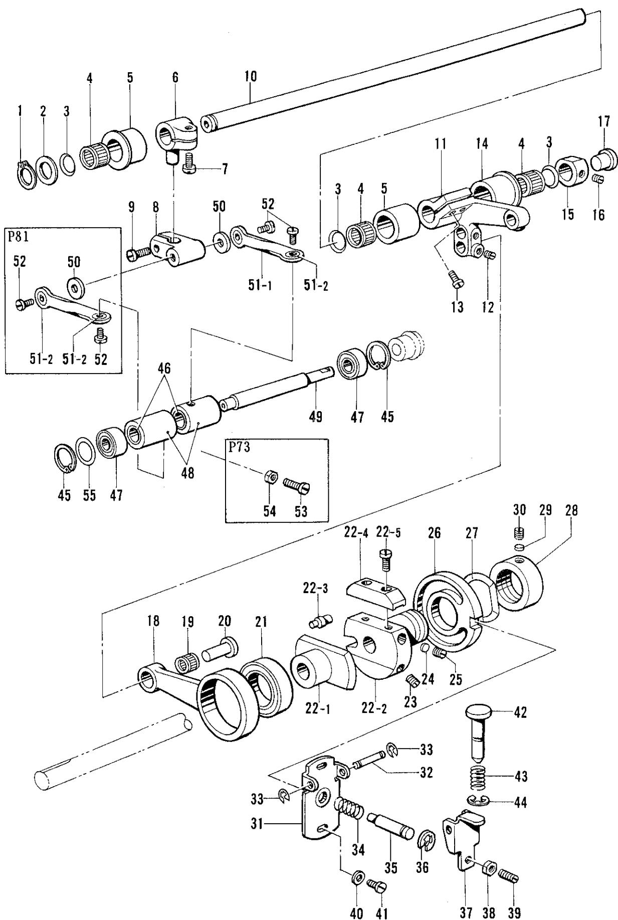
D. 送り関係/Feed mechanism/Transportvorrichtung/
