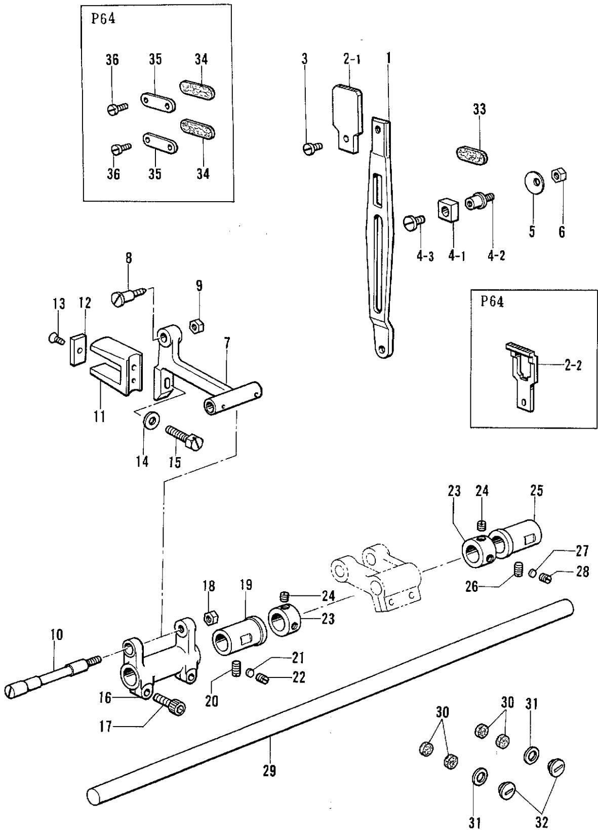
G. 送り軸関係/Feed shaft mechanism/Transport welle/
