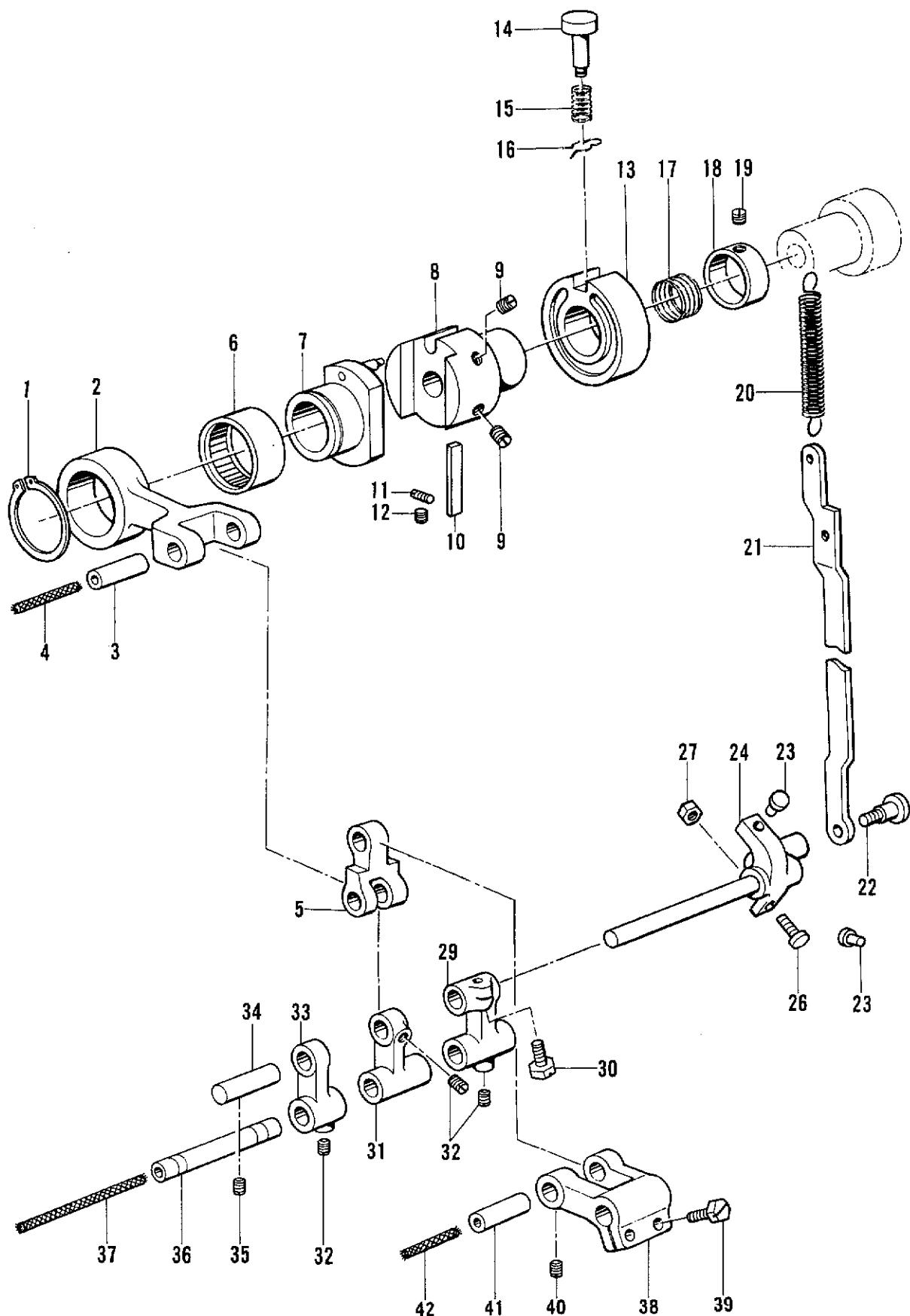
F. 送り関係/Feed mechanism/Transportvorrichtung/
