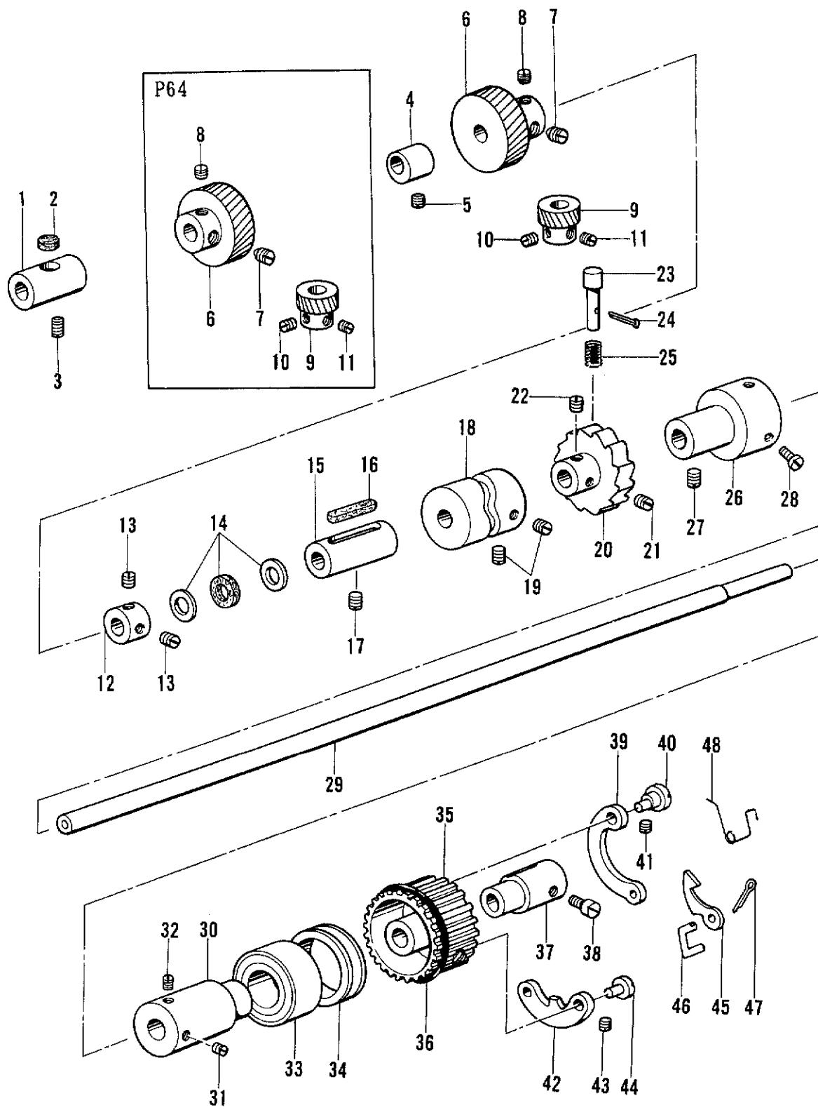
H. 下軸関係/Lower shaft mechanism/Untere Welle/
