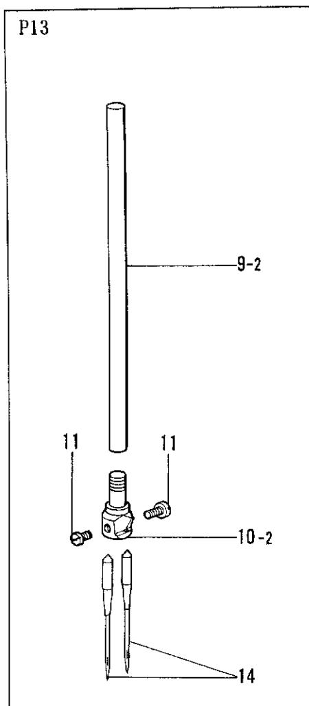
C. 針棒関係/Needle bar mechanism/Nadelstangenvorrichtung/
