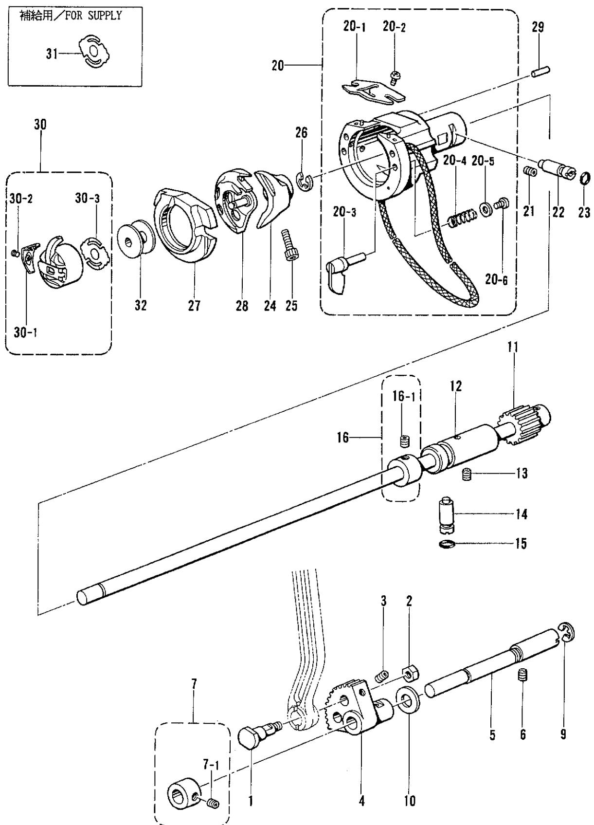
G. 下軸関係/Lower shaft mechanism/Untere Welle/
