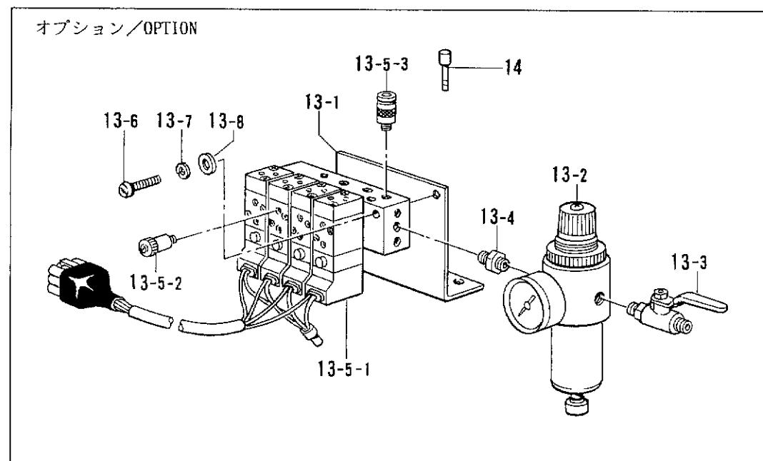
**U. 空圧関係/Air pressure mechanism/Luftdruck/
