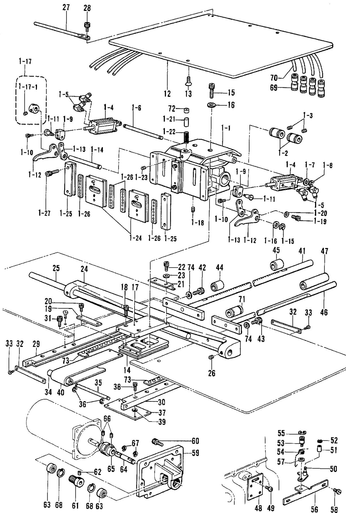
D1. 送り関係/Feed mechanism (1)/Transportvorrichtung (1)/
