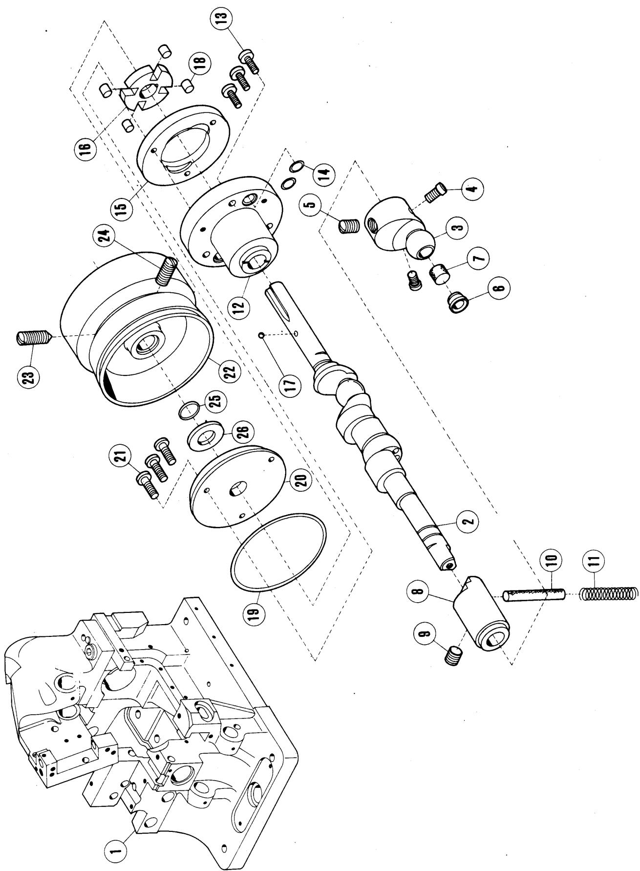
**MACHINE FRAME, CRANKSHAFT & OIL PUMPING MECHANISM**
