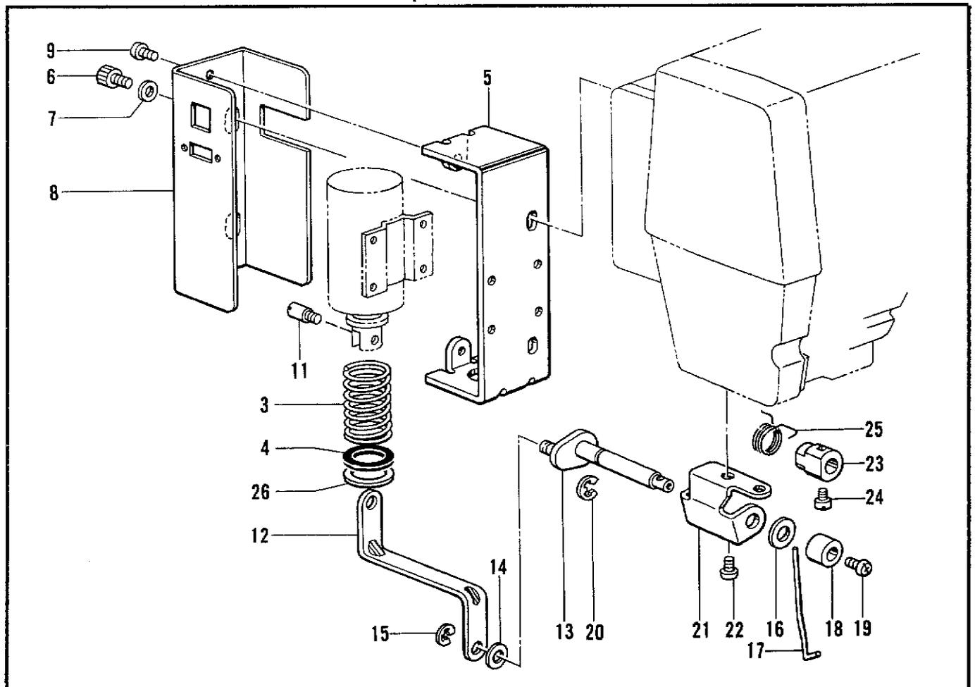
M. 糸切れ感知関係/Thread breakage detector mechanism/Fadenbruchfühler/
