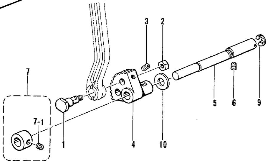
G. 下軸関係/Lower shaft mechanism/Untere Welle/
