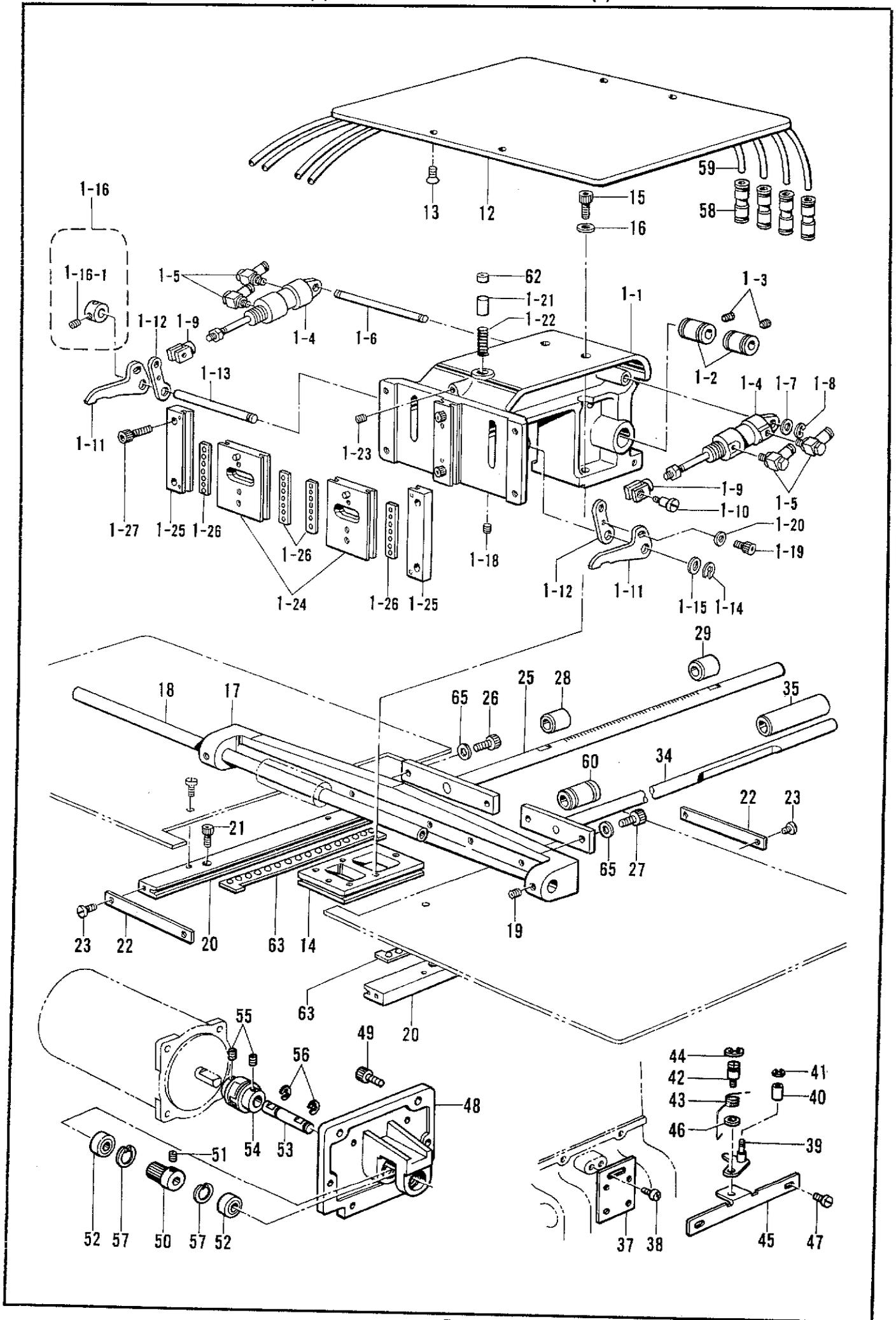
D1. 送り関係/Feed mechanism (1)/Transportvorrichtung (1)/
