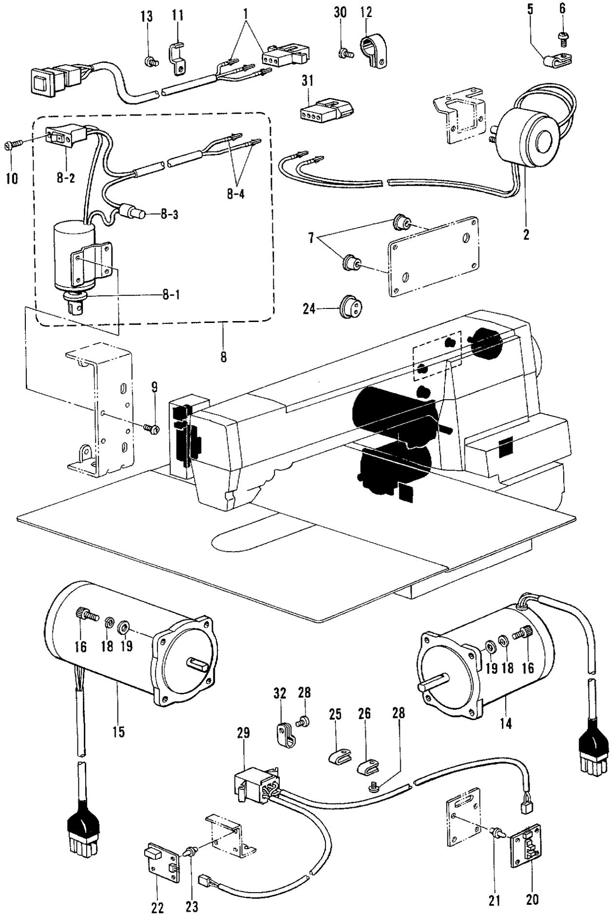
Q. 電装品関係 / Power supply equipment mechanism / Stromversorgung /
