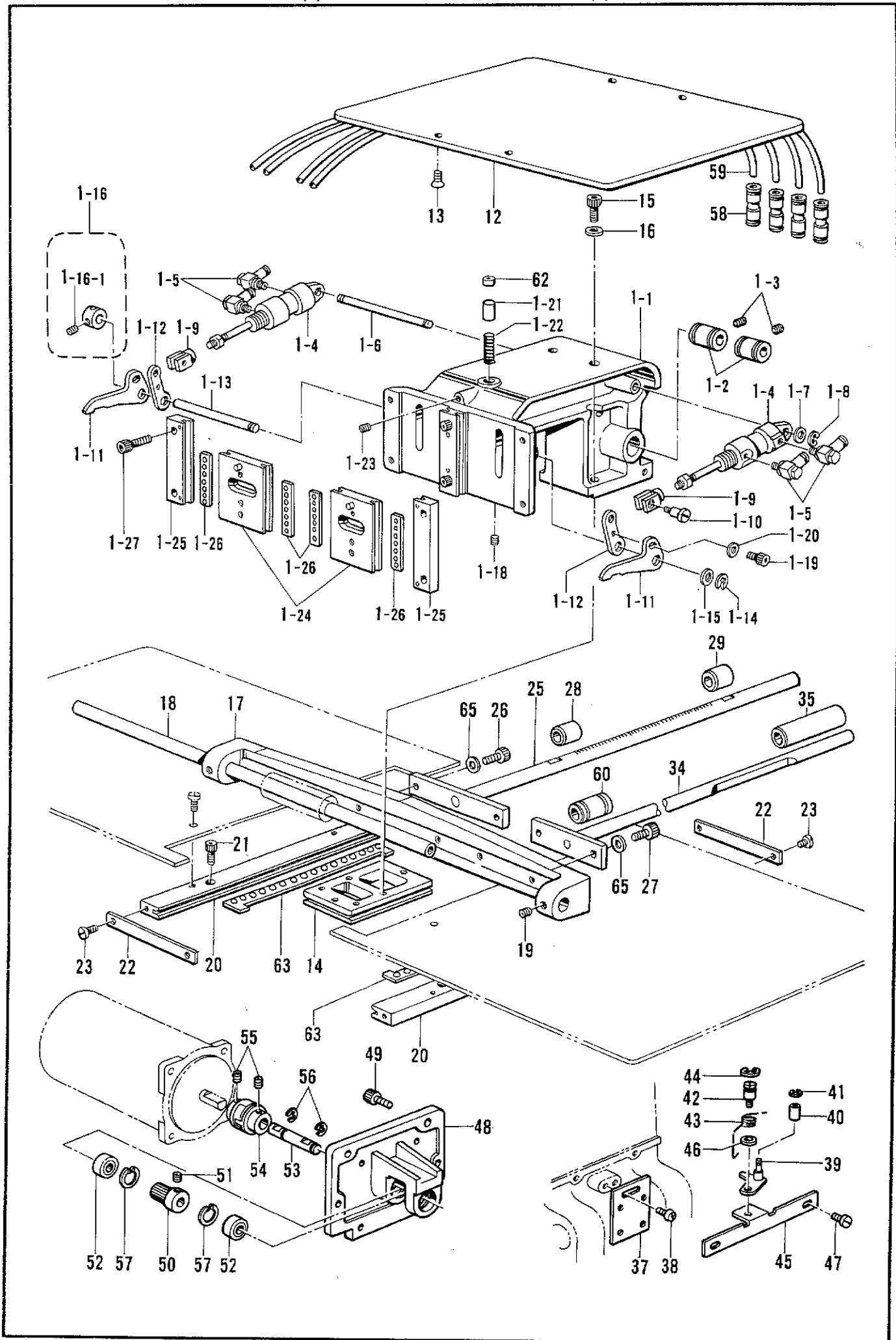
D1. 送り関係/Feed mechanism (1)/Transportvorrichtung (1)/
