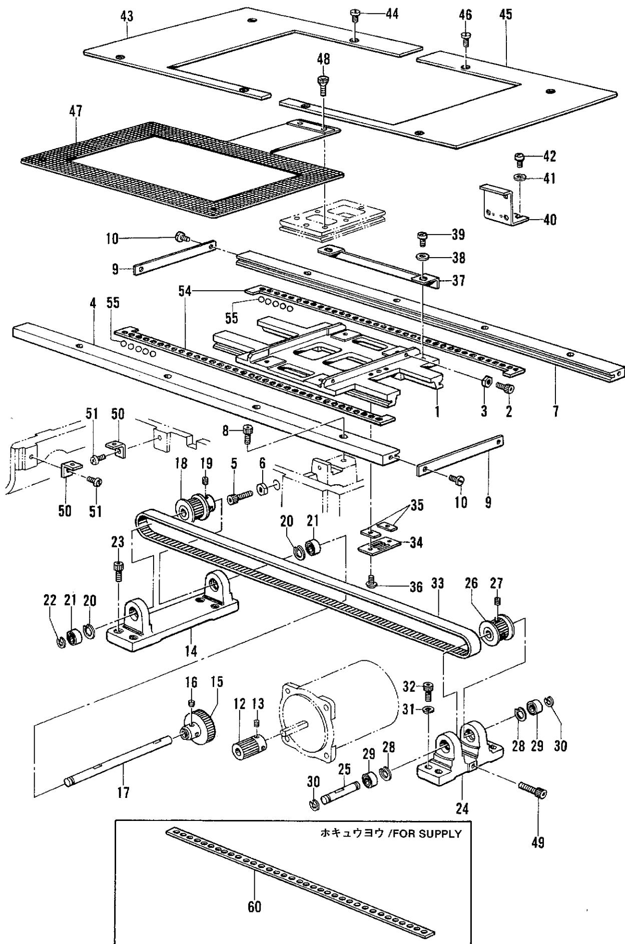
F. 駆動側送り関係 /Feed guide mechanism/Transportführung/
