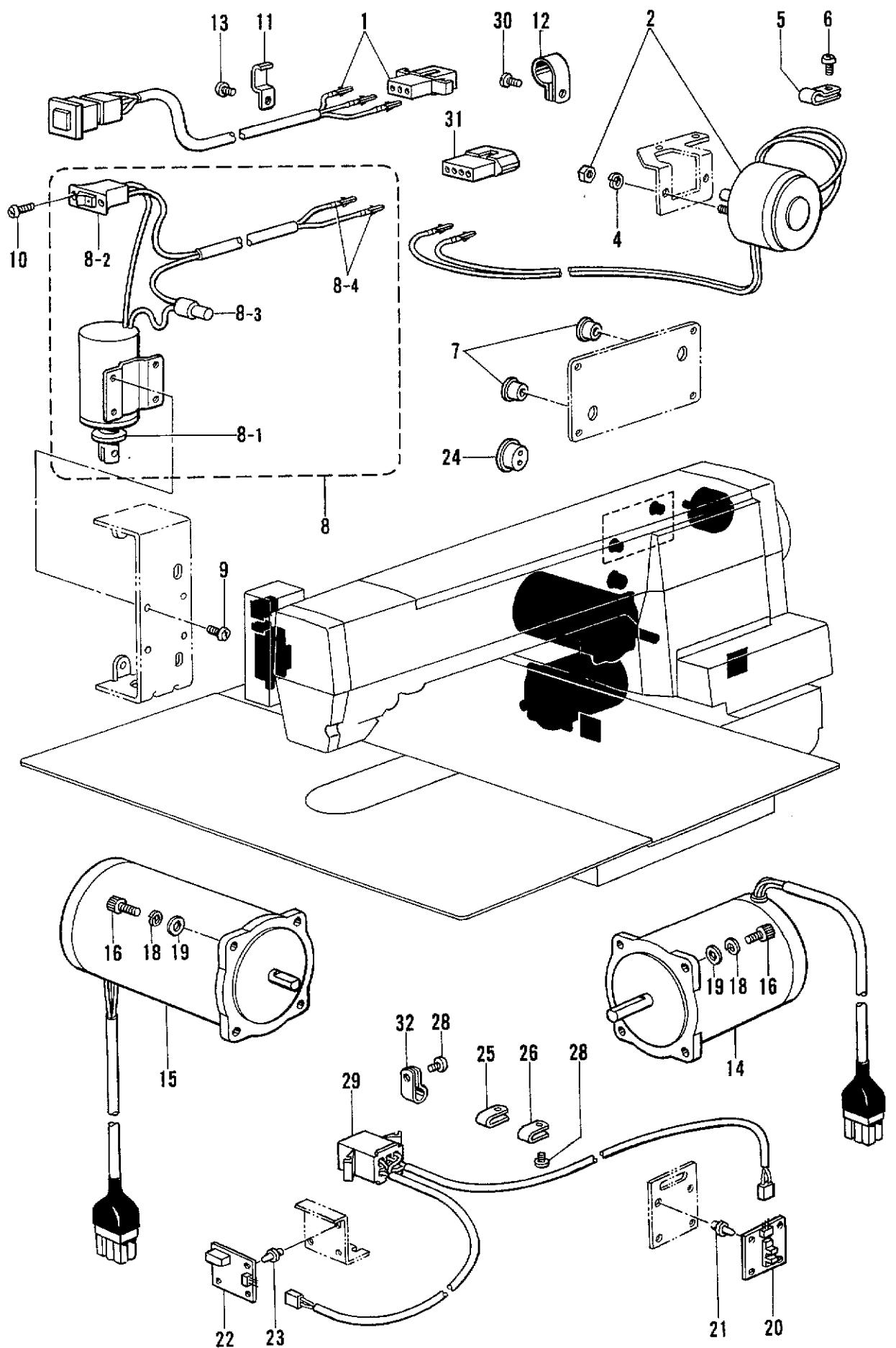
Q. 電装品関係/Power supply equipment mechanism/Stromversorgung/
